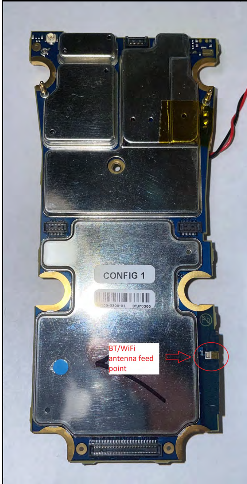
BT/Wi-Fi Antenna Feed Point
