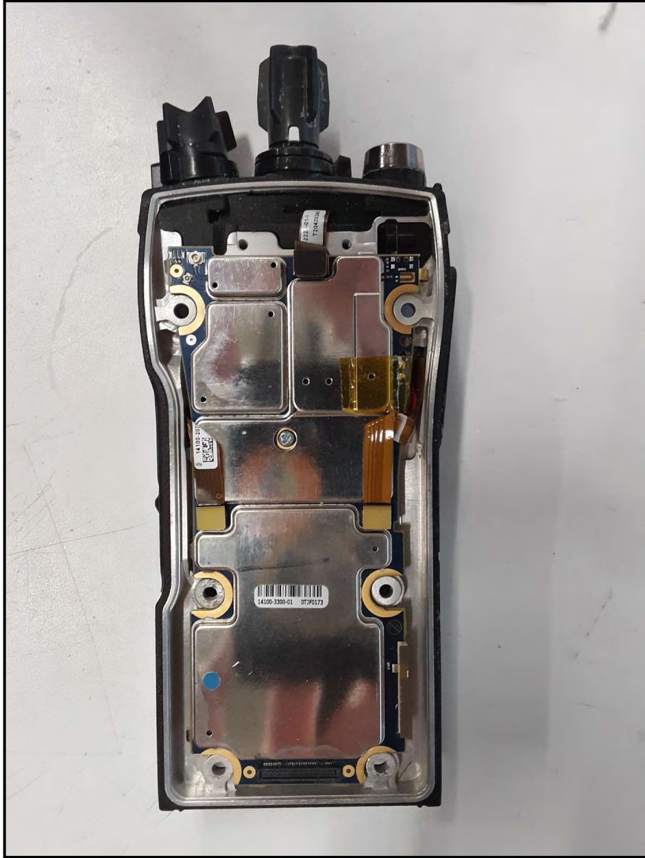
Main Board Installed in Chassis
