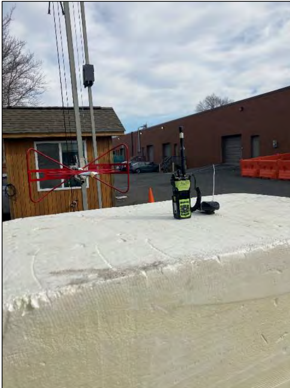
Photograph 4: Radiated Emissions – Back View (Above 1 GHz)
