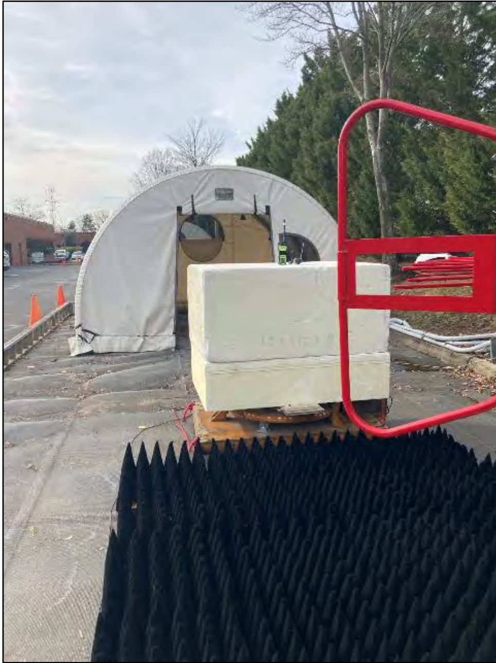
Photograph 3: Radiated Emissions – Front View (Above 1 GHz)
