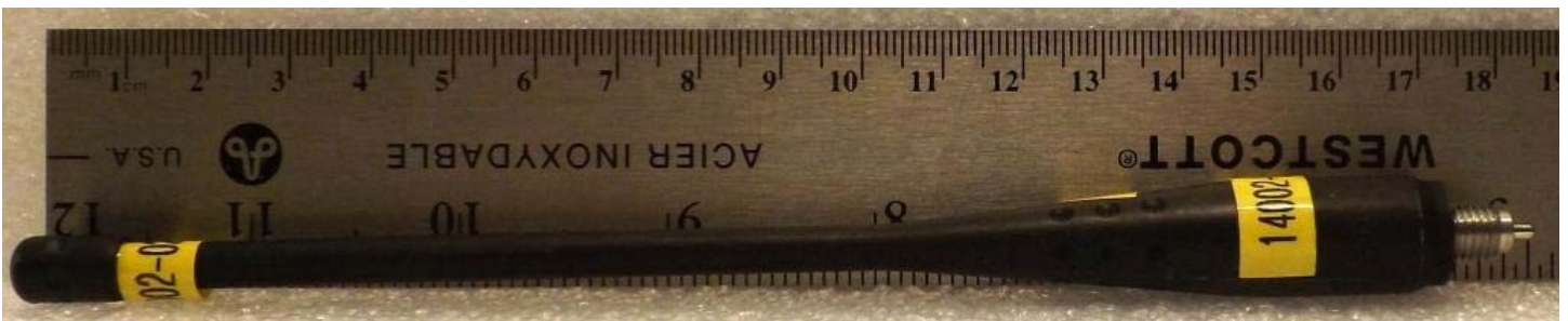
Figure D.14– T4 – 14002-0223-01 Antenna
