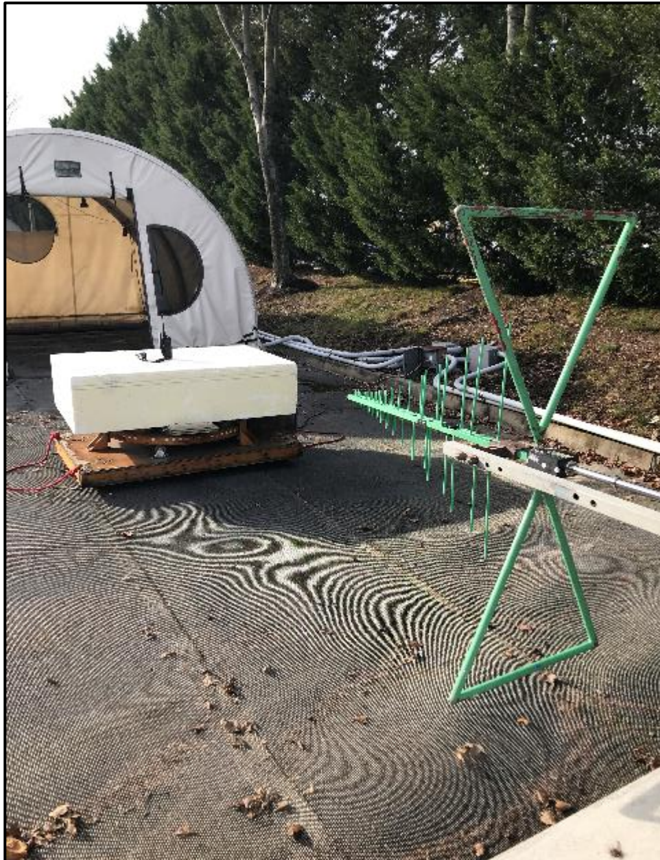
Photograph 3: Radiated Emissions Testing – Front View (Below 1 GHz)
