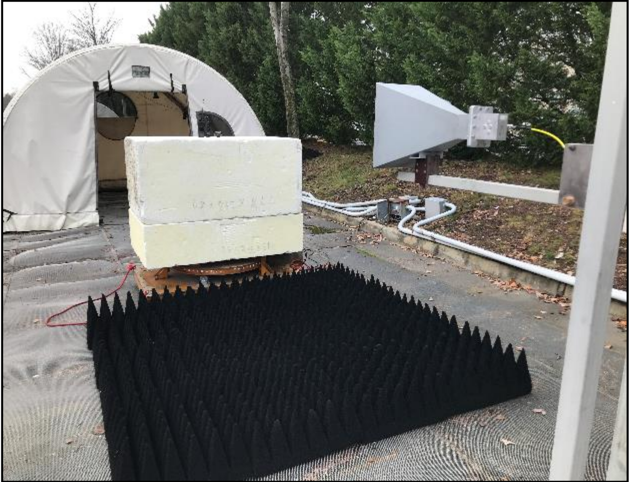
Photograph 1: Radiated Emissions Testing – Front View (Above 1 GHz)
