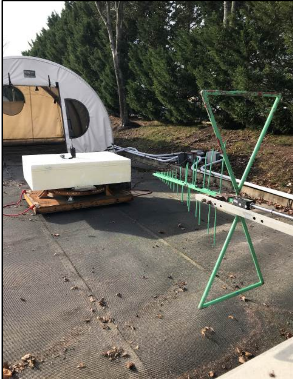
Photograph 3: Radiated Emissions Testing – Front View (Below 1 GHz)
