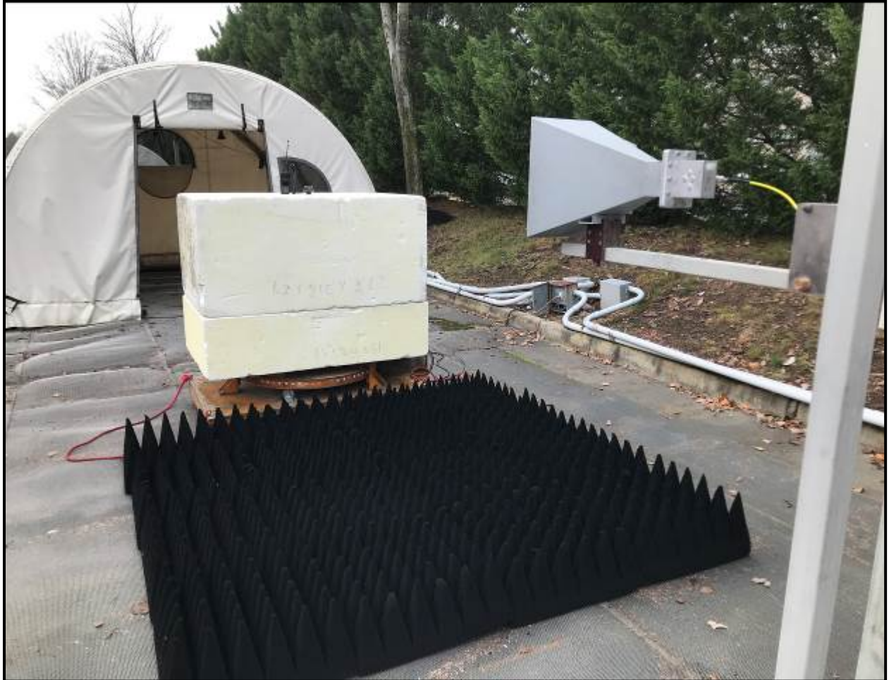
Photograph 1: Radiated Emissions Testing – Front View (Above 1 GHz)
