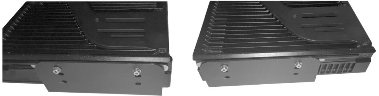
Figure 8-9: Acceptable VCH Positions within Bracket
