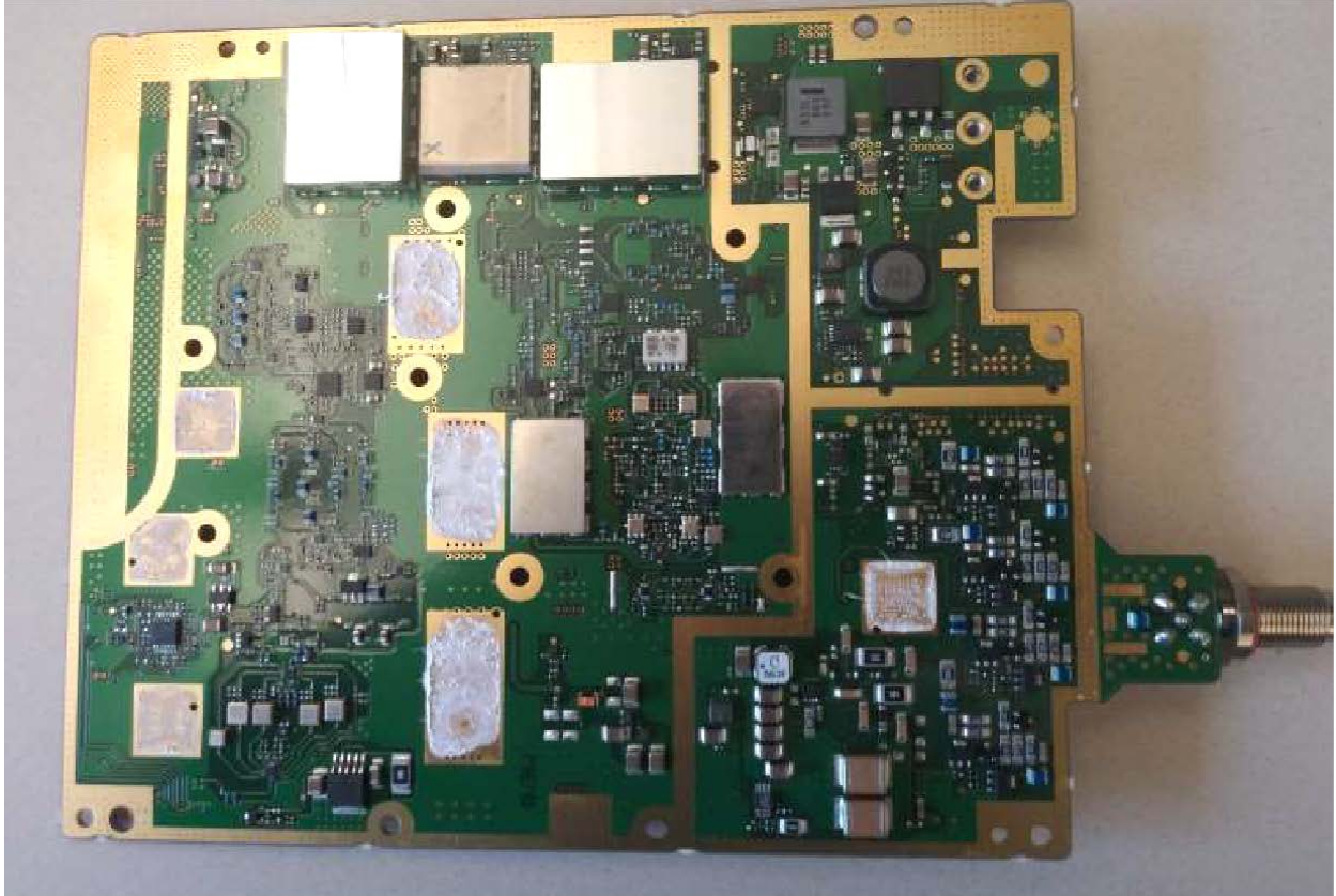
VCH RF Board Solder Side with Shields
