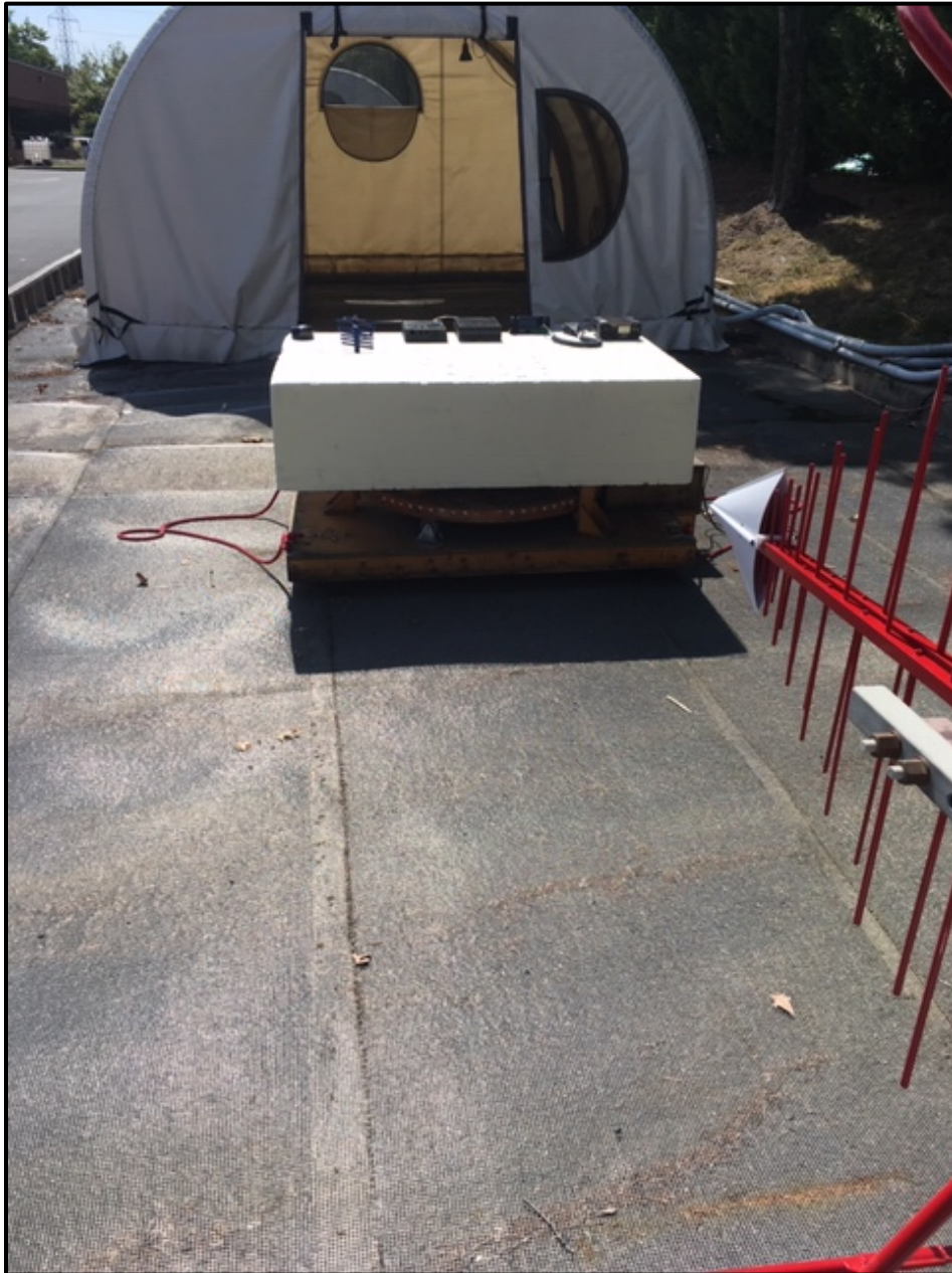
Photograph 3: Radiated Emissions Testing – Front View (Below 1 GHz)
