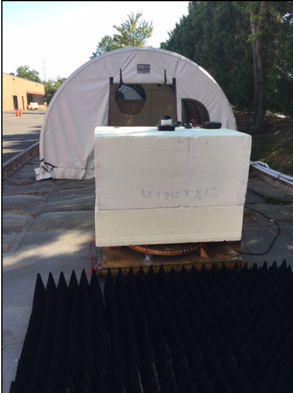
Photograph 1: Radiated Emissions Testing – Front View (Above 1 GHz)
