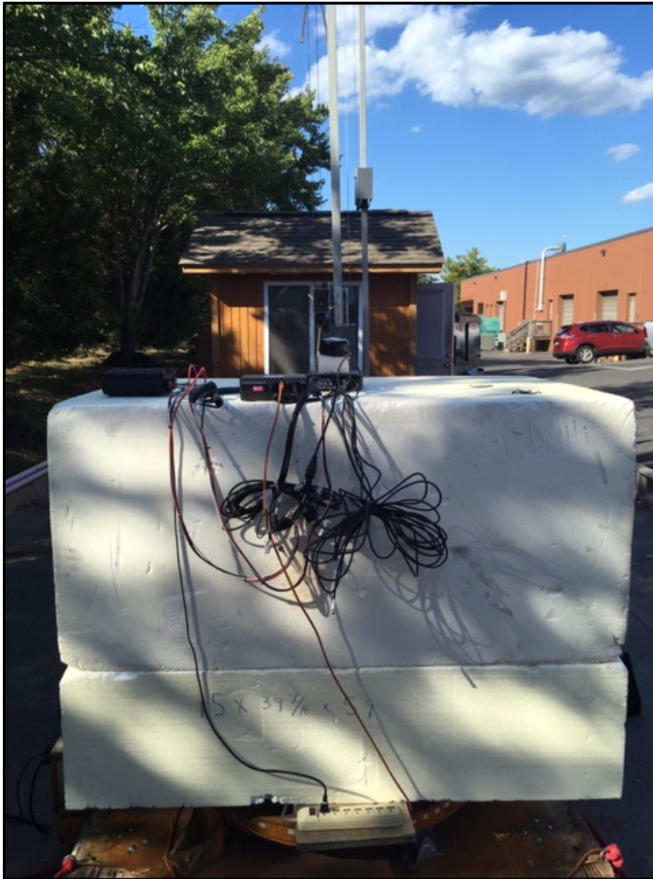
Photograph 2: Radiated Emissions Testing – Back View (Above 1 GHz)
