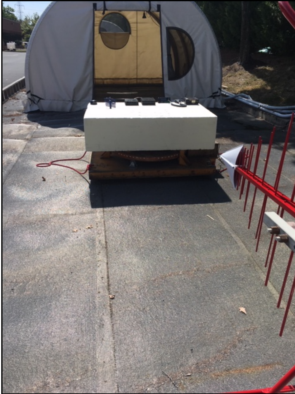
Photograph 3: Radiated Emissions Testing – Front View (Below 1 GHz)
