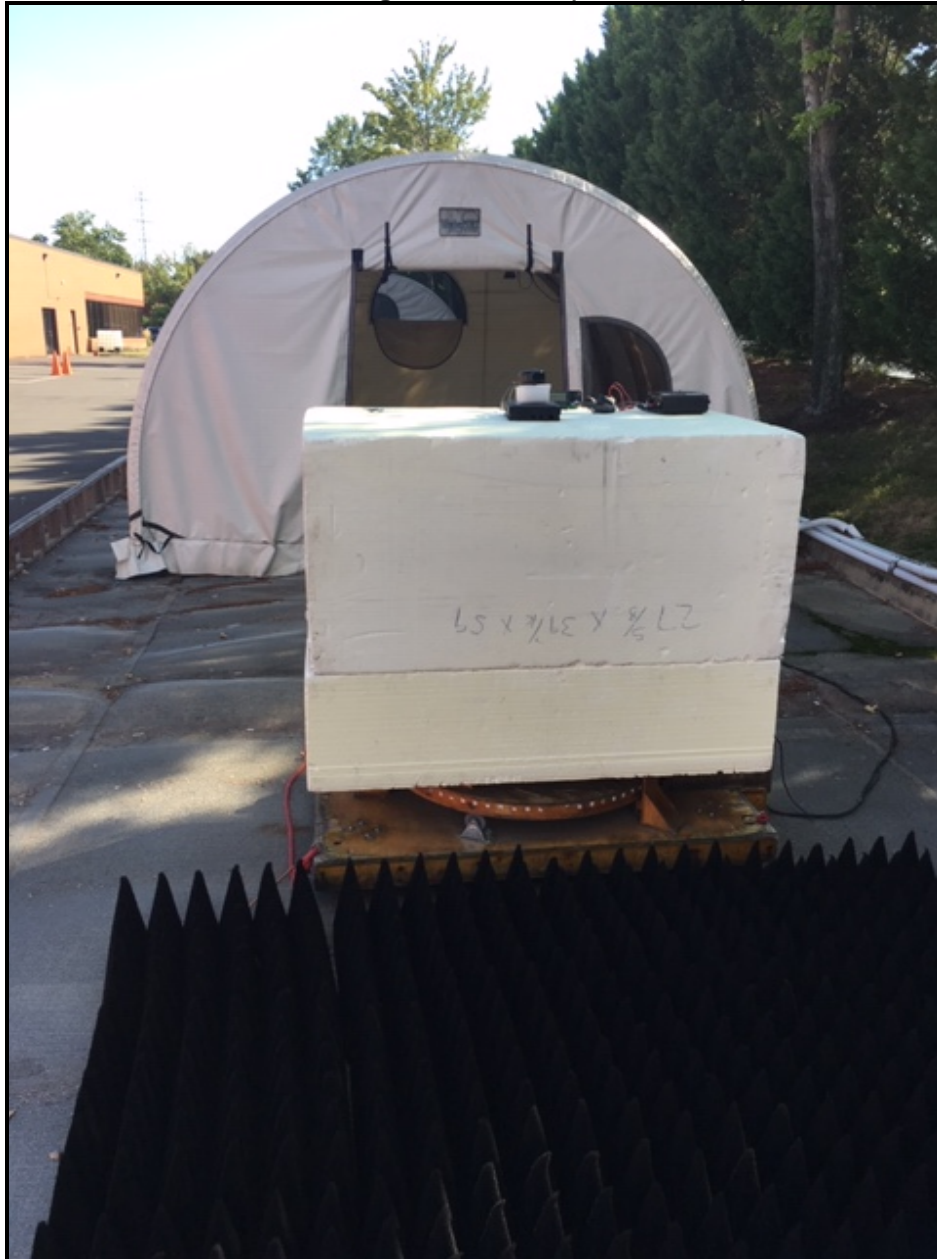
Photograph 1: Radiated Emissions Testing – Front View (Above 1 GHz)
