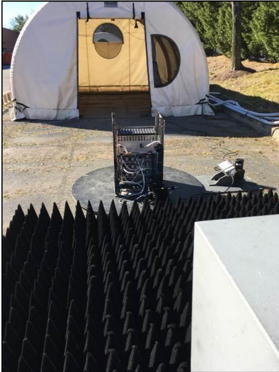
Photograph 2: Radiated Emissions (Spurious/Harmonics) – Back View (Above 1 GHz)
