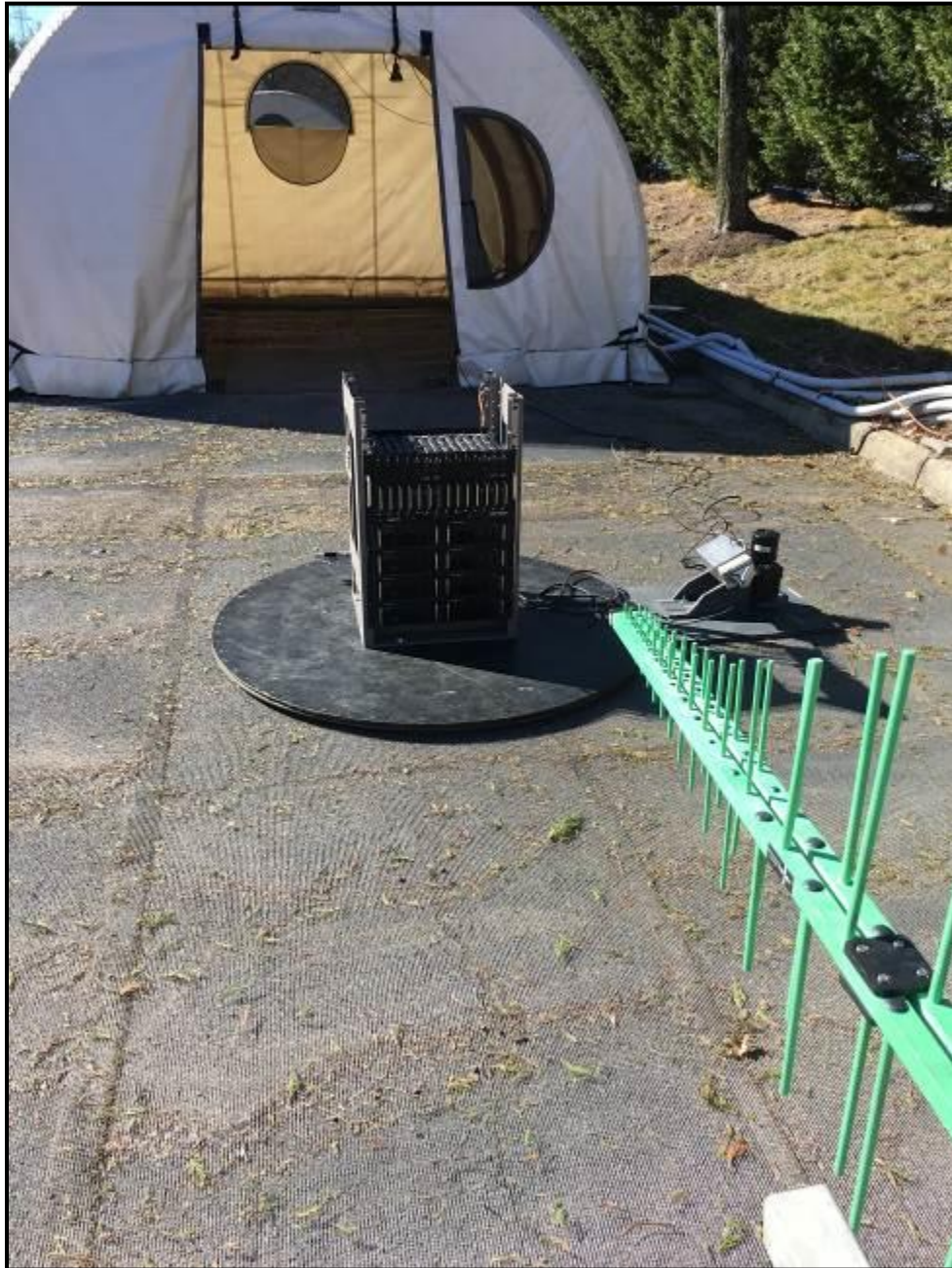
Photograph 3: Radiated Emissions (Spurious/Harmonics) – Front View (Below 1 GHz)
