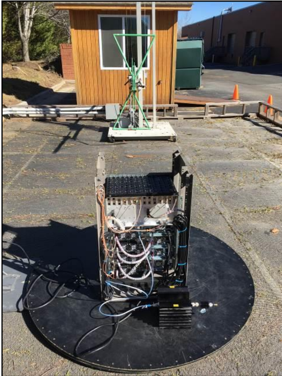
Photograph 4: Radiated Emissions (Spurious/Harmonics) – Back View (Below 1 GHz)
