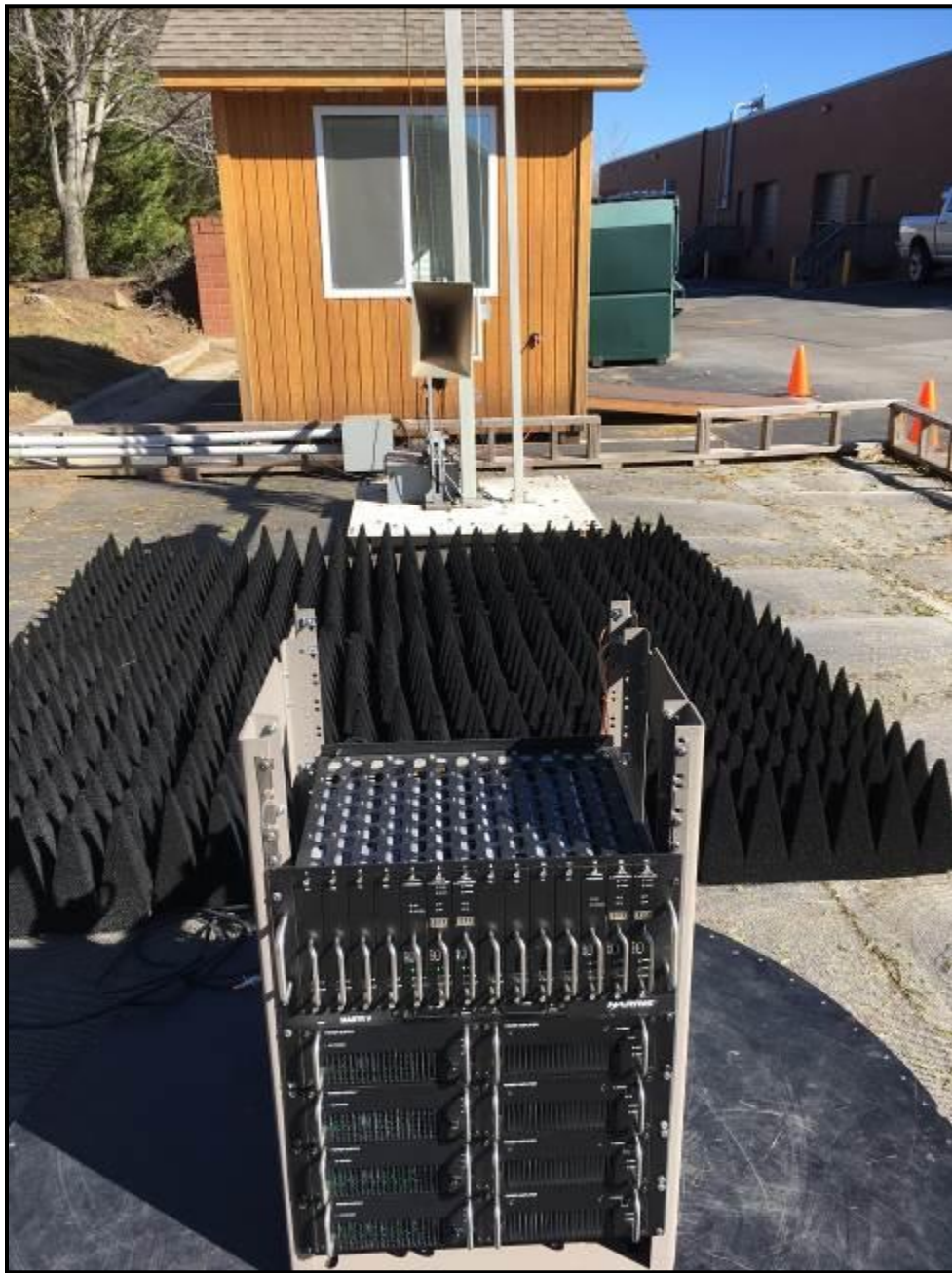
Photograph 1: Radiated Emissions (Spurious/Harmonics) – Front View (Above 1 GHz)
