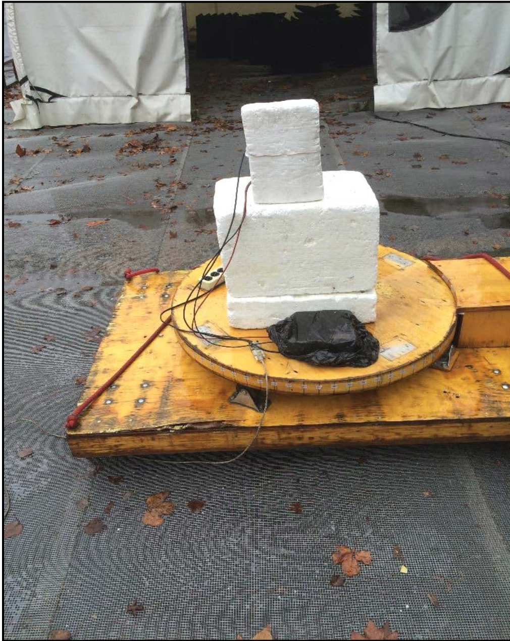
Photograph 4: Radiated Emissions Testing – Back View <1 GHz
