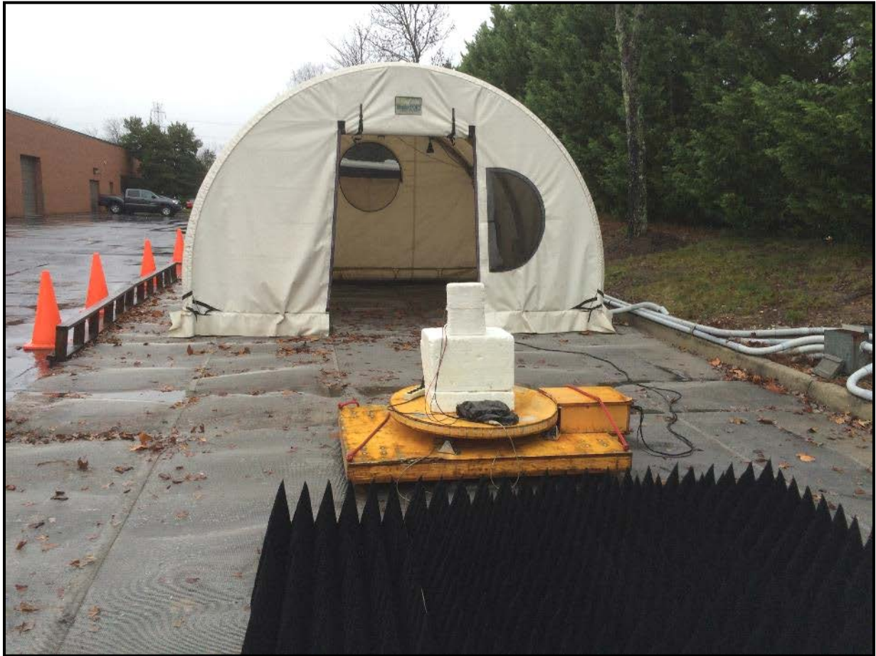
Photograph 2: Radiated Emissions Testing – Back View >1 GHz
