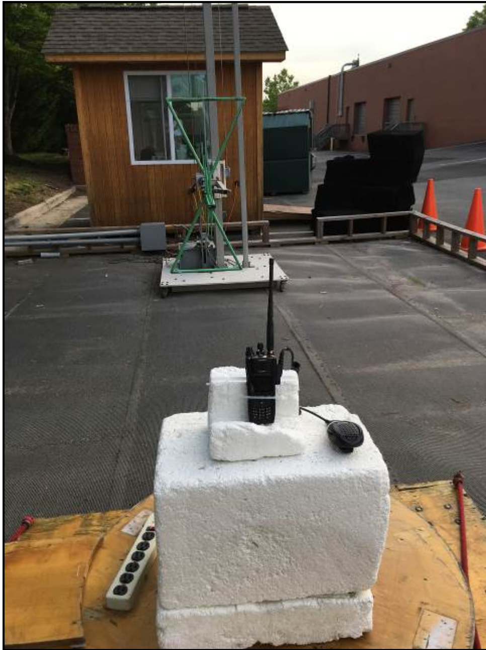
Photograph 1: Radiated Emissions – Front View, <1 GHz
