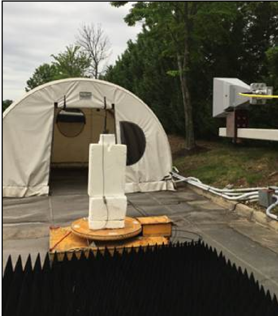
Photograph 4: Radiated Emissions – Back View, >1GHz
