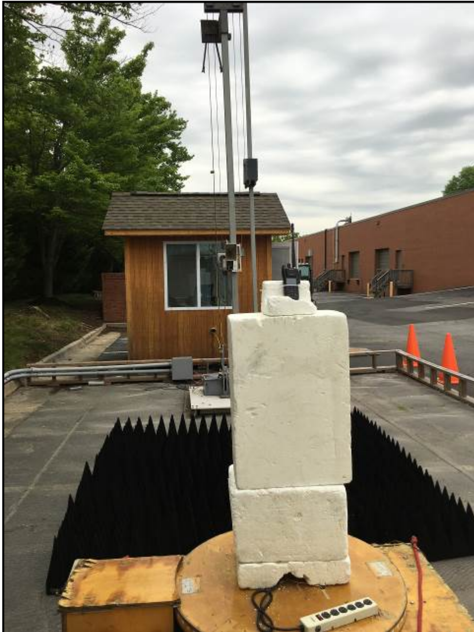
Photograph 3: Radiated Emissions – Front View, >1 GHz
