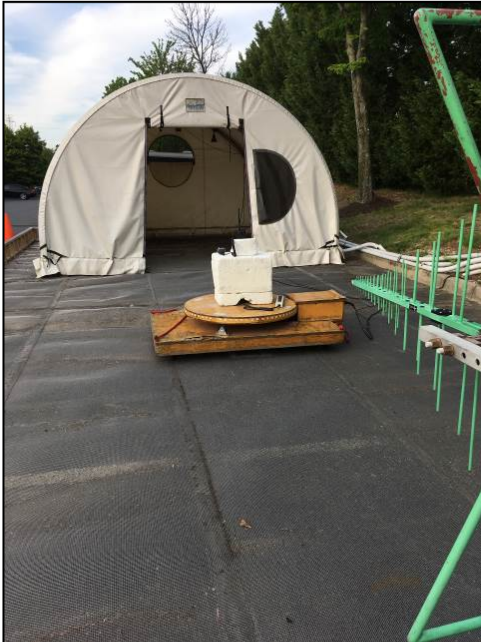
Photograph 2: Radiated Emissions – Back View, <1GHz
