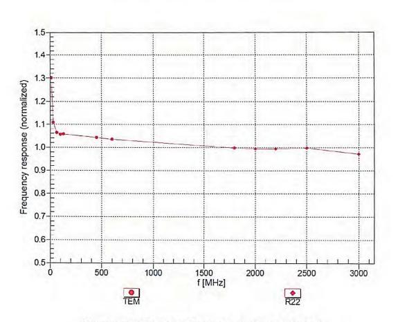
Frequency Response of E-Field (TEM-Cell:ifi110 EXX, Waveguide: R22)
