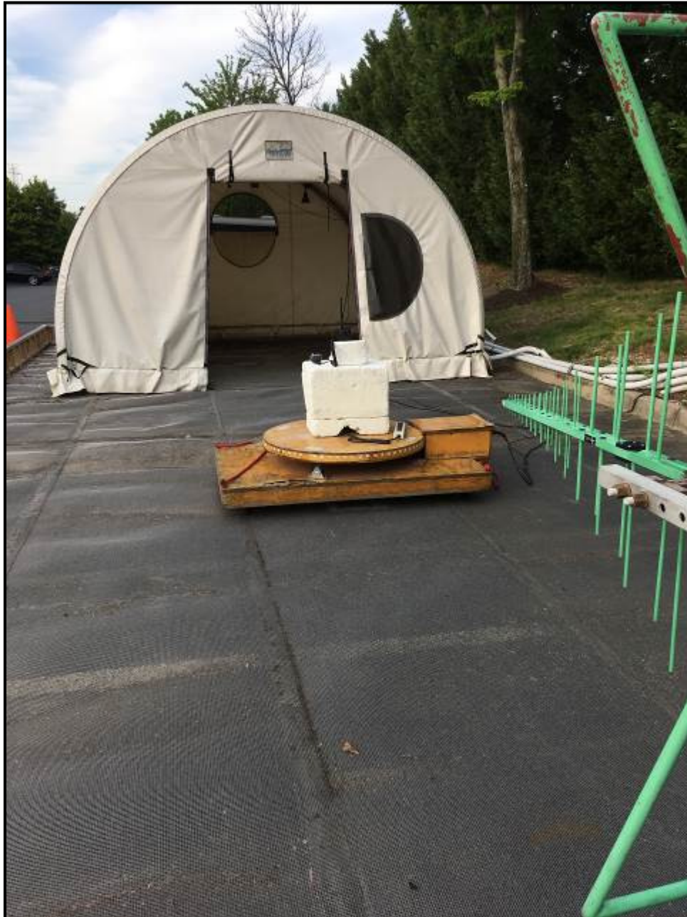
Photograph 2: Radiated Emissions – Back View, <1GHz
