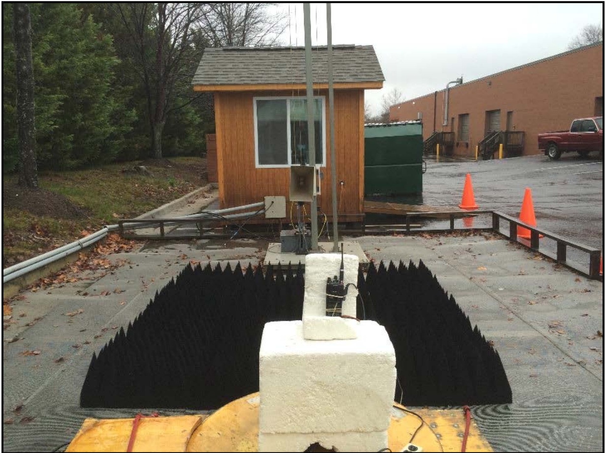
Photograph 1: Radiated Emissions Testing – Front View >1 GHz
