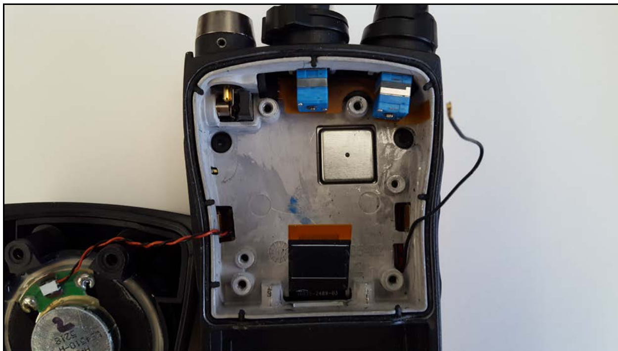
Rear Cover and Expansion Board Removed
