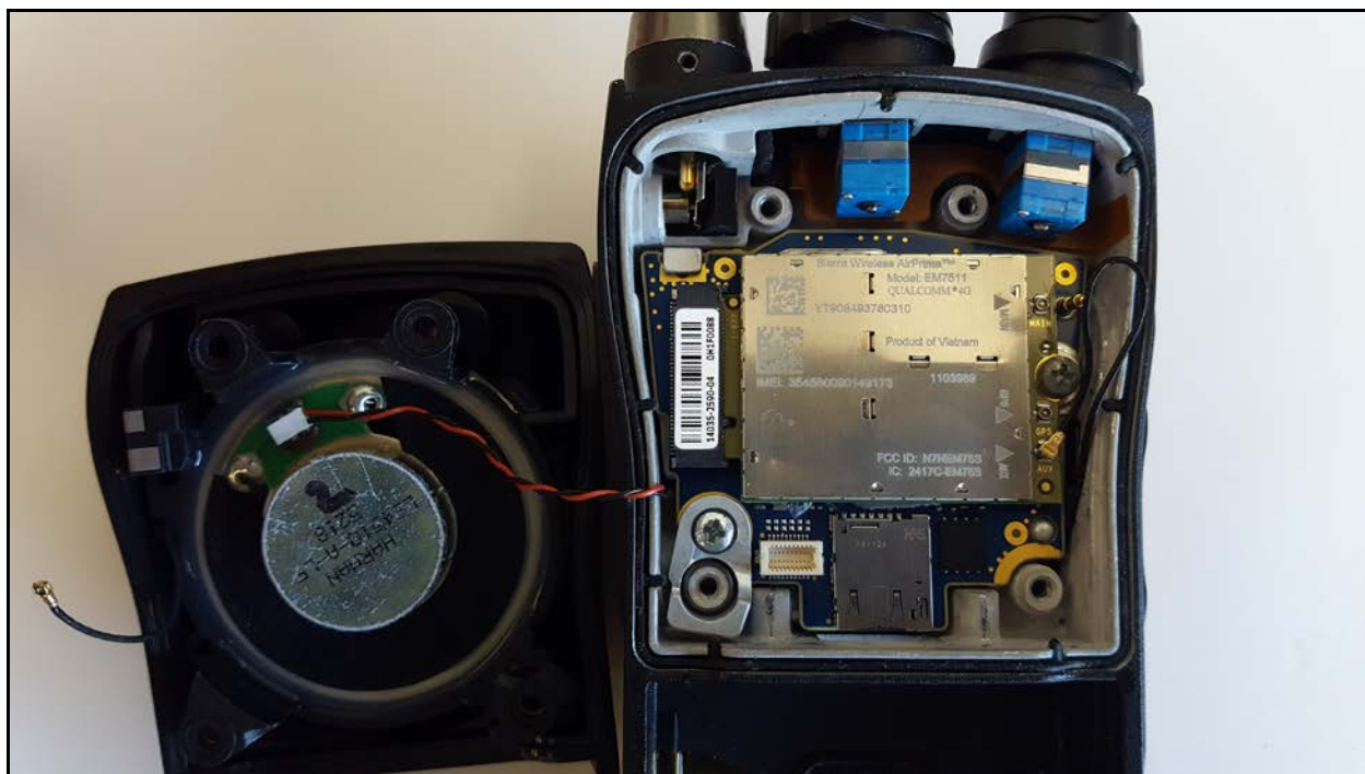
Rear Cover and Grounding Strap Removed; LTE Module
