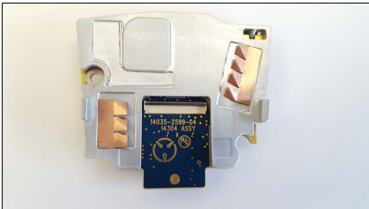
Expansion Board with LTE Module and LTE Processor Shield - Bottom
