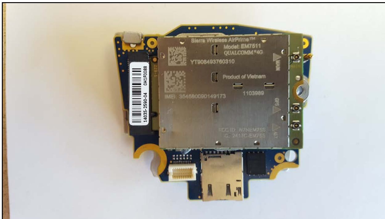
Expansion Board with LTE Module and LTE Processor Shield - Top
