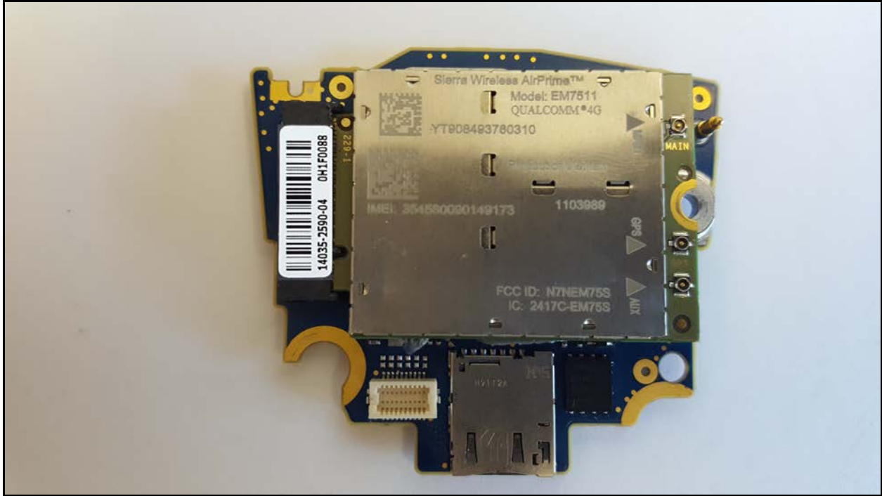
Expansion Board with LTE Module and no LTE Processor Shield – Top
