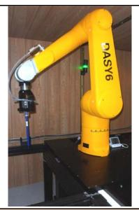
**DASY 6 SAR System with SAM Phantom**
