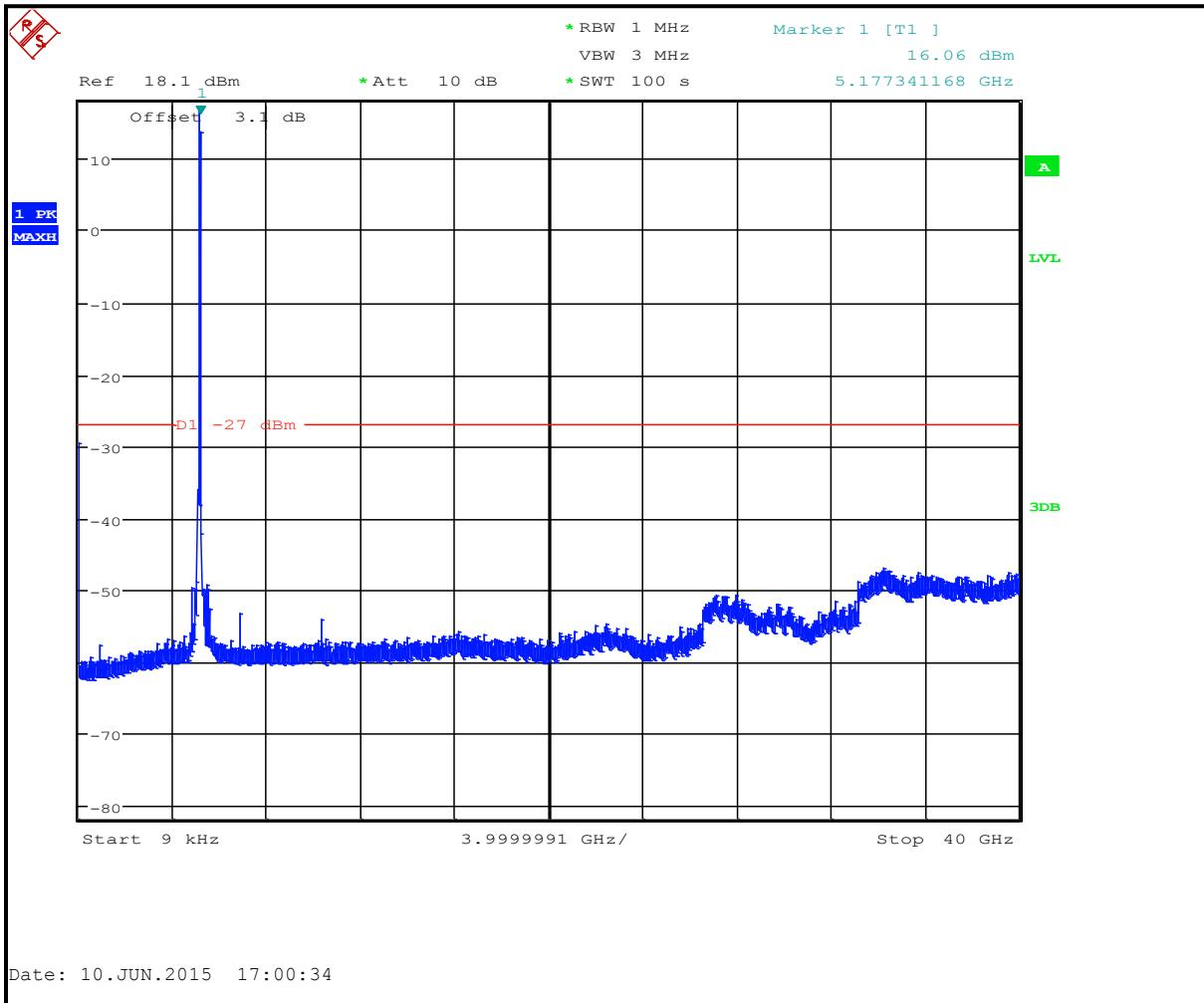
**Plot 7-4: Undesirable Emissions Channel 40 (5200 MHz)**
