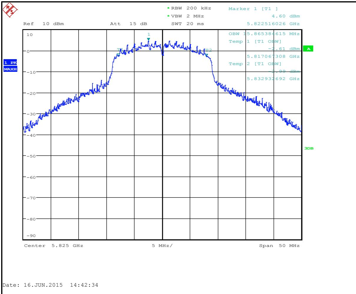
**Plot 8-56: 6 dB Bandwidth Channel 149 (TX Frequency 5745 MHz) - 802.11n**
