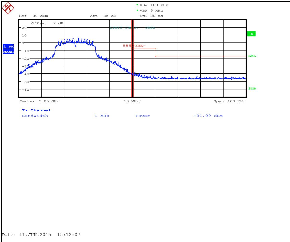
**Note:** Conducted antenna port measurement
