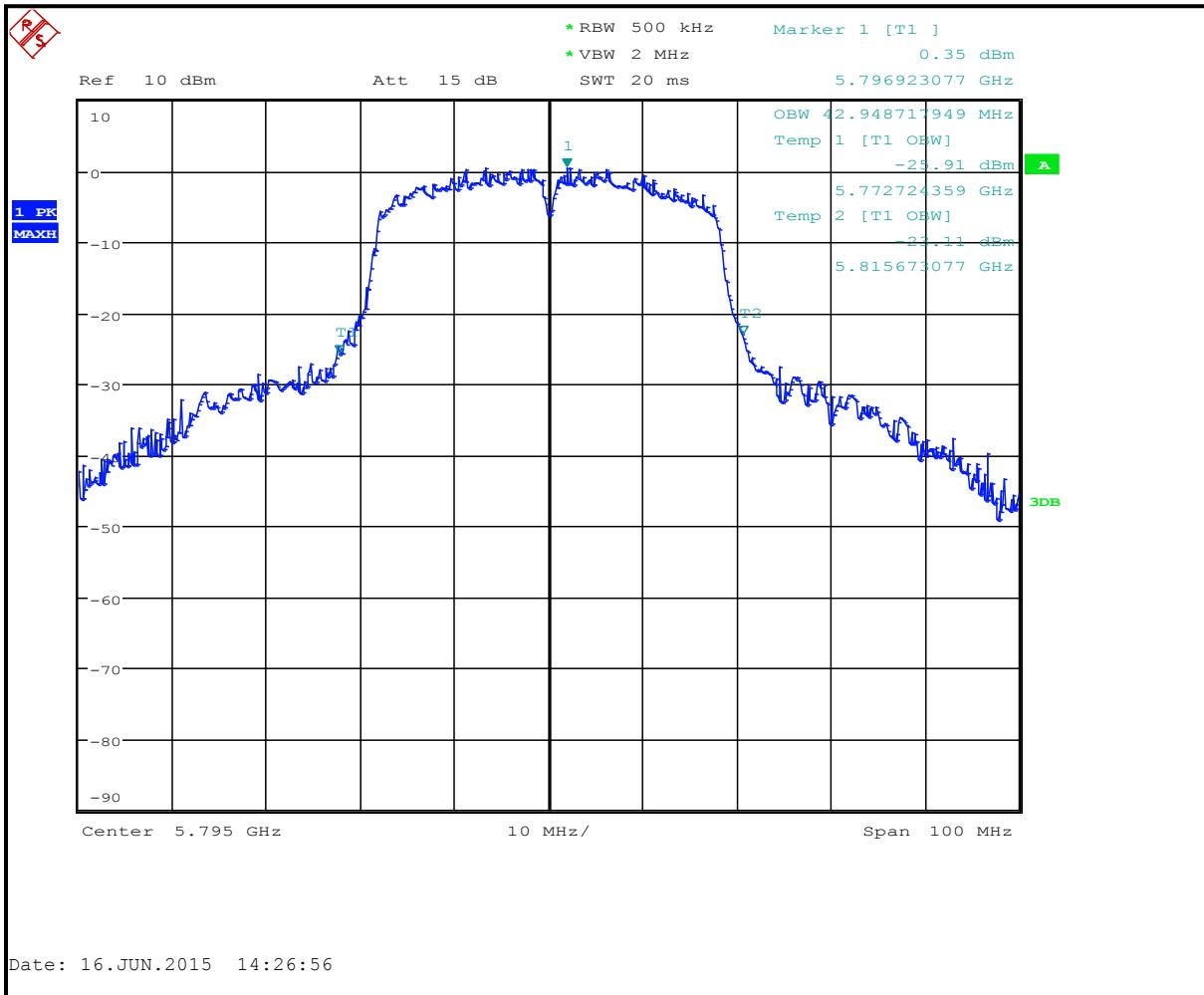
**Plot 8-52: 26 dB Bandwidth (Frequency 5815 MHz) - 802.11n (40 MHz BW)**
