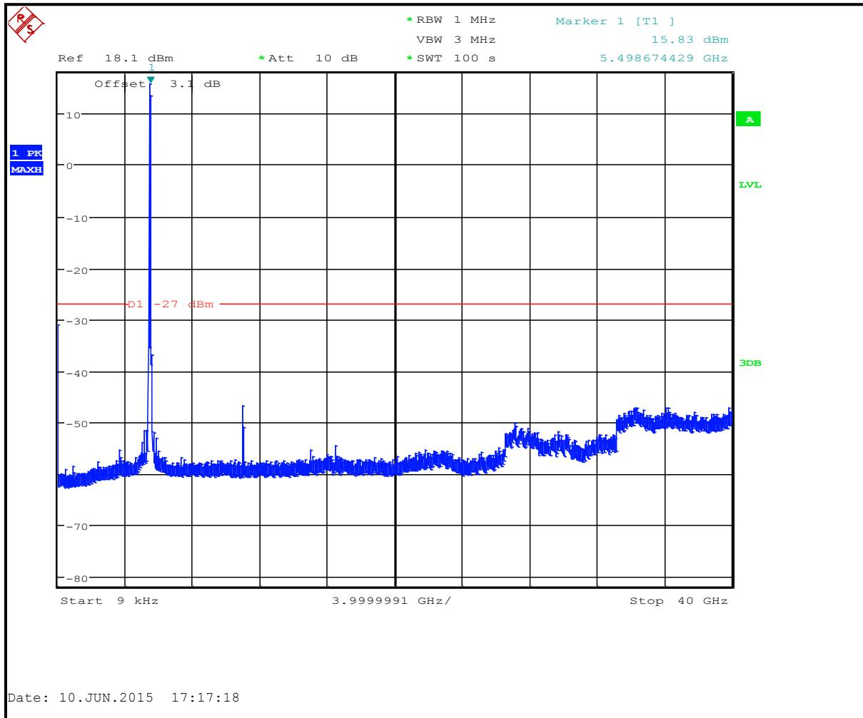
**Plot 7-11: Undesirable Emissions Channel 116 (5580 MHz)**
