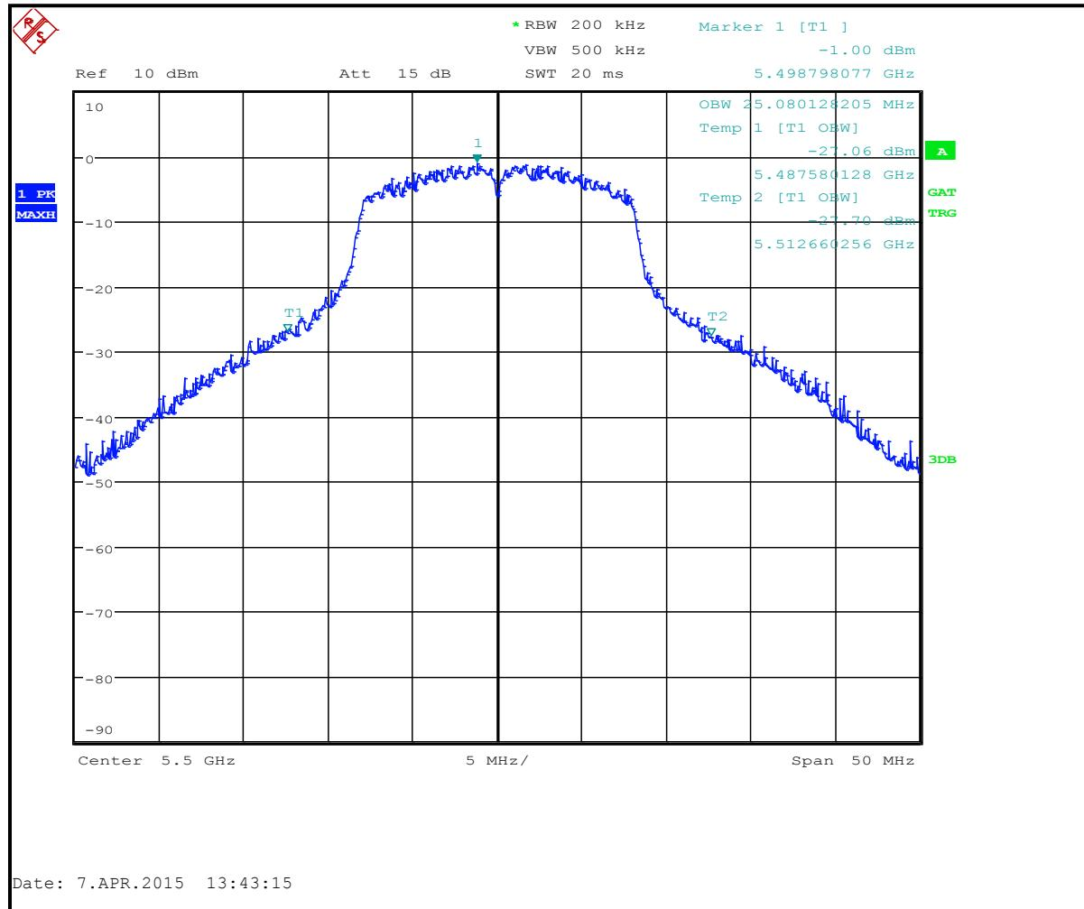
**Plot 8-22: 26 dB Bandwidth Channel 116 (TX Frequency 5580 MHz) - 802.11n**
