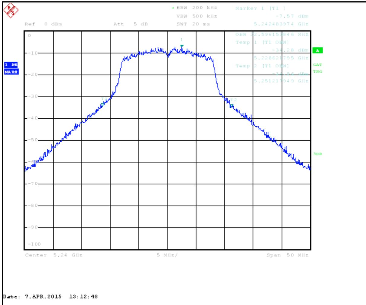
**Plot 8-18: 26 dB Bandwidth Channel 52 (TX Frequency 5260 MHz) - 802.11n**
