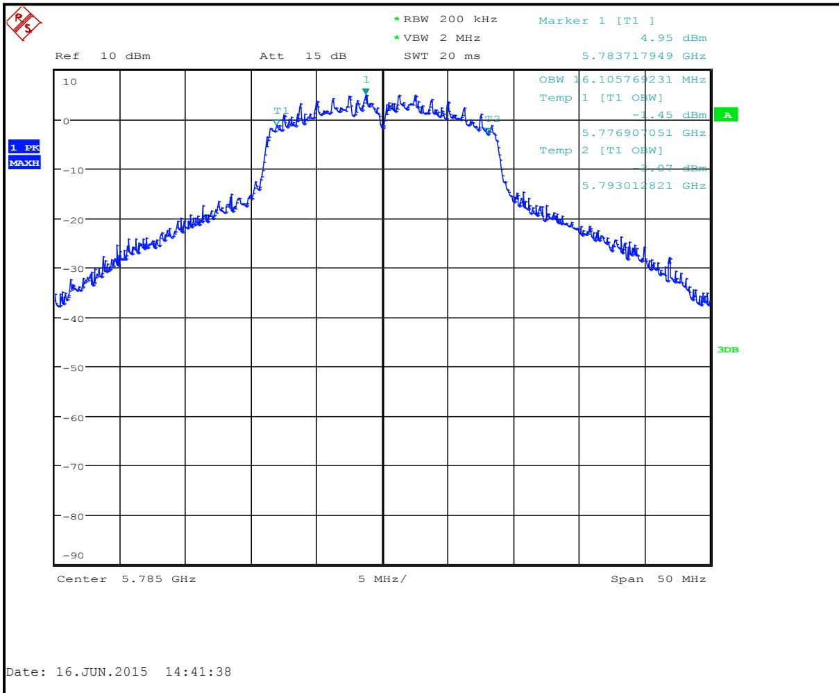
**Plot 8-55: 6 dB Bandwidth Channel 165 (TX Frequency 5825 MHz) - 802.11a**
