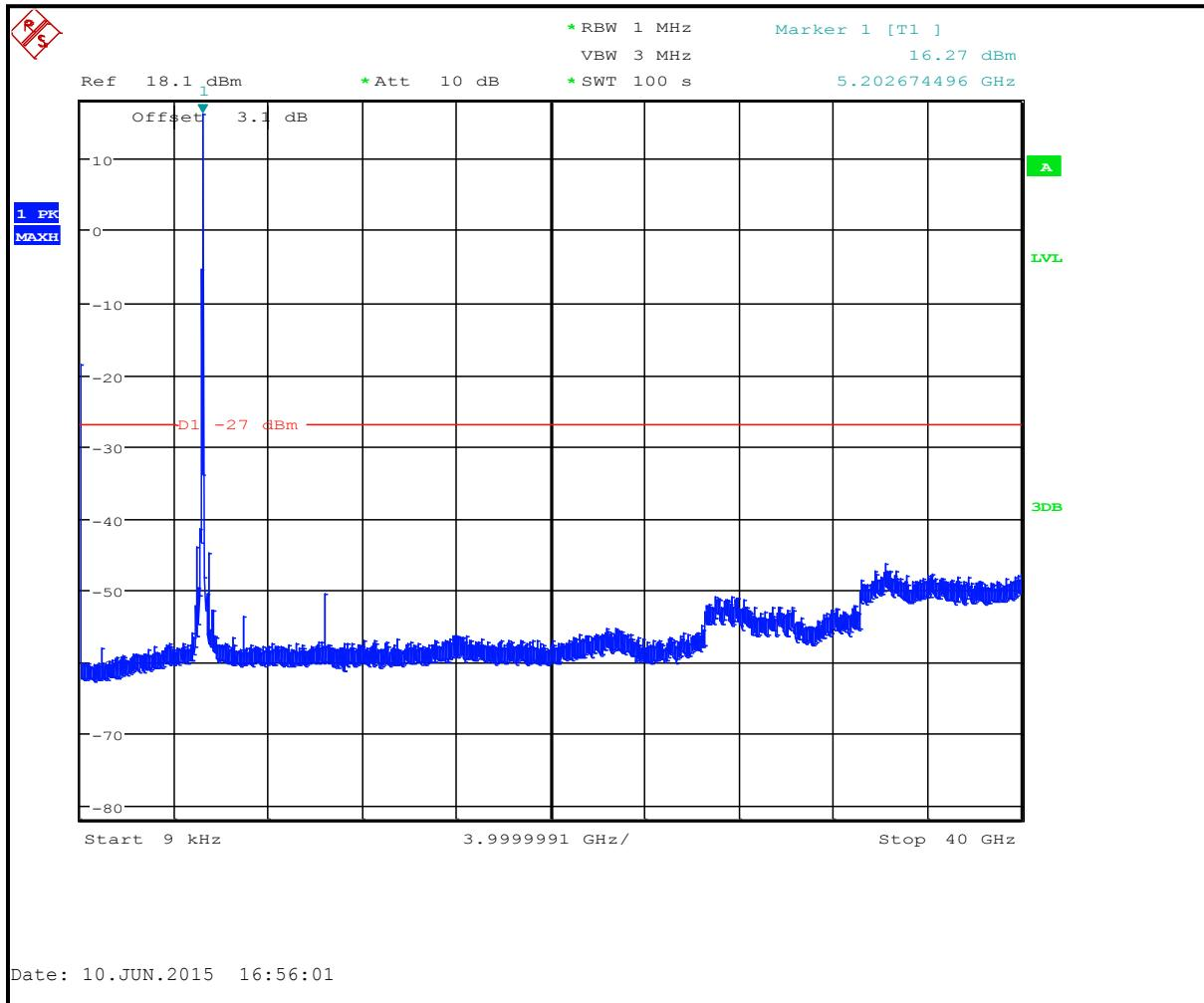
**Plot 7-5: Undesirable Emissions Channel 44 (5220 MHz)**
