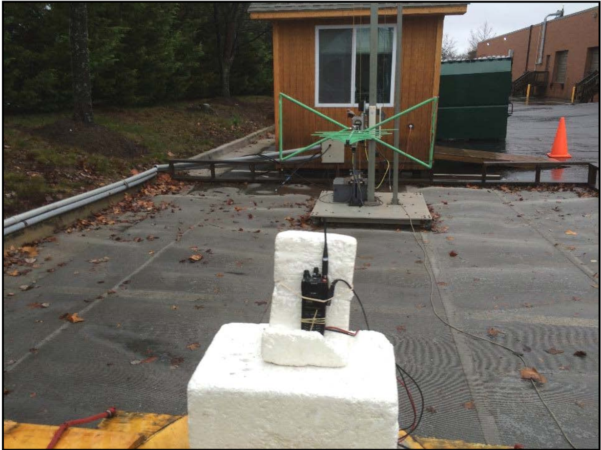
Photograph 3: Radiated Emissions Testing – Front View <1 GHz
