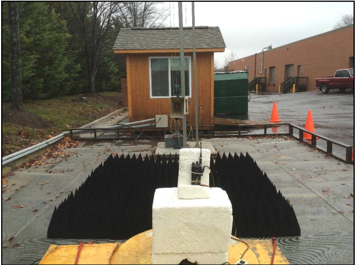
Photograph 1: Radiated Emissions Testing – Front View >1 GHz
