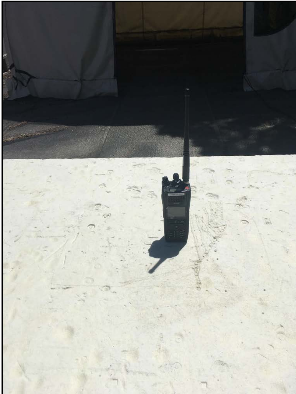
Photograph 3: Radiated Emissions (Spurious/Harmonics) Under 1 GHz, Front View
