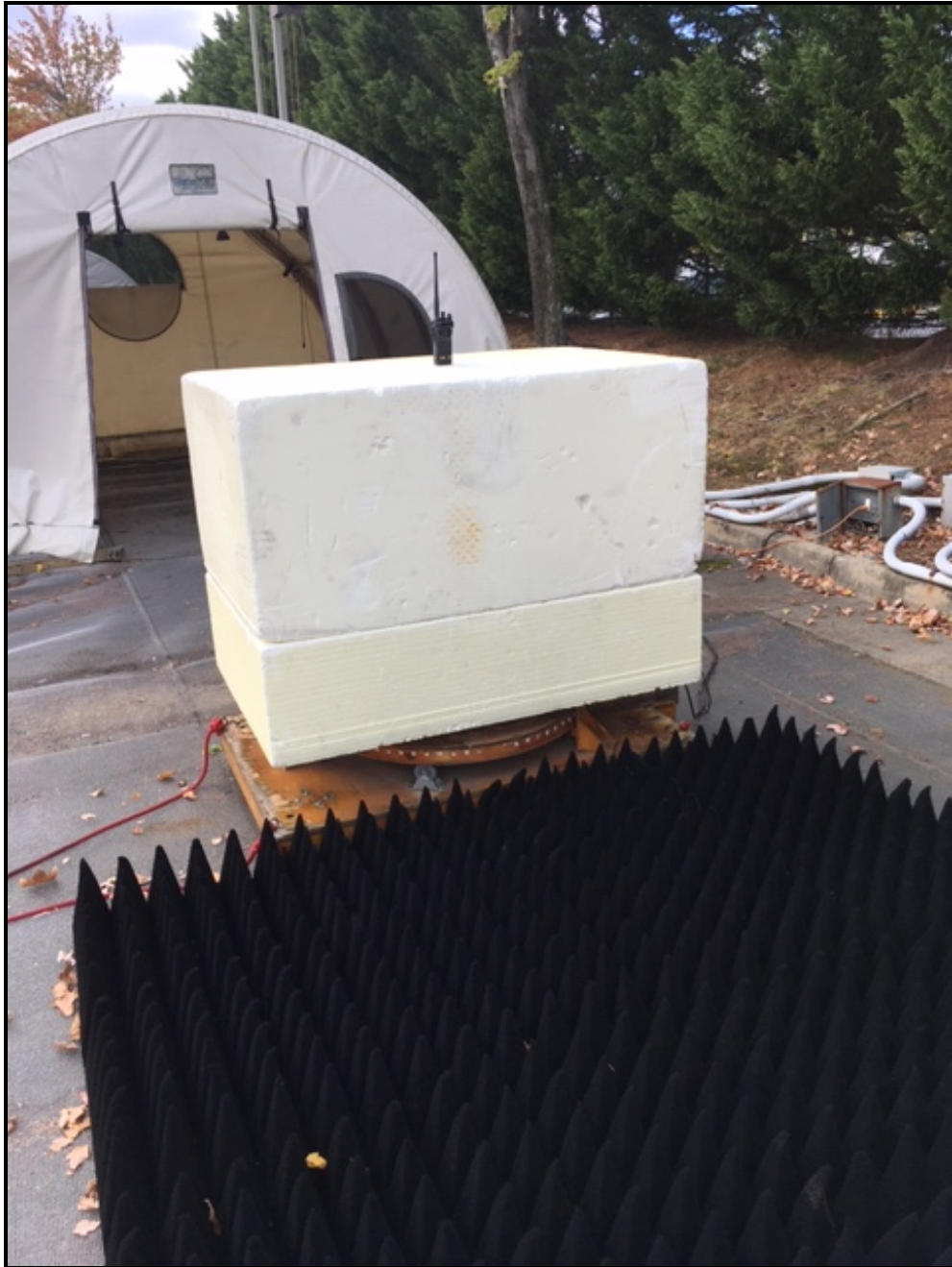
Photograph 2: Radiated Emissions (Spurious/Harmonics) Over 1 GHz, Back View
