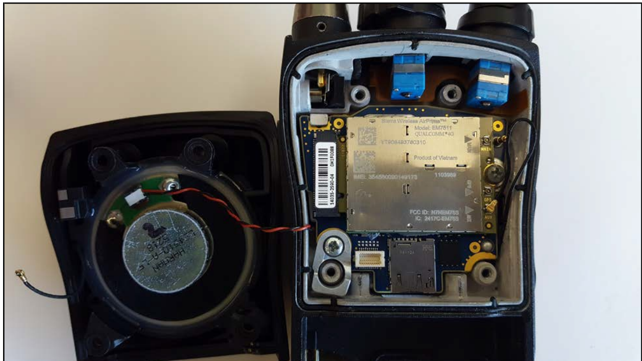
Rear Cover and Grounding Strap Removed; LTE Module
