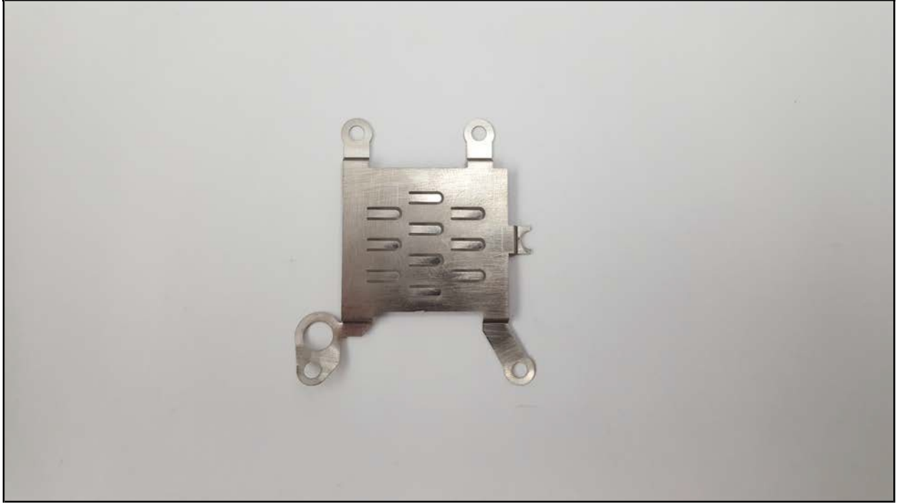
Grounding Strap – Top
