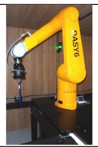
**DASY 6 SAR System with SAM Phantom**
