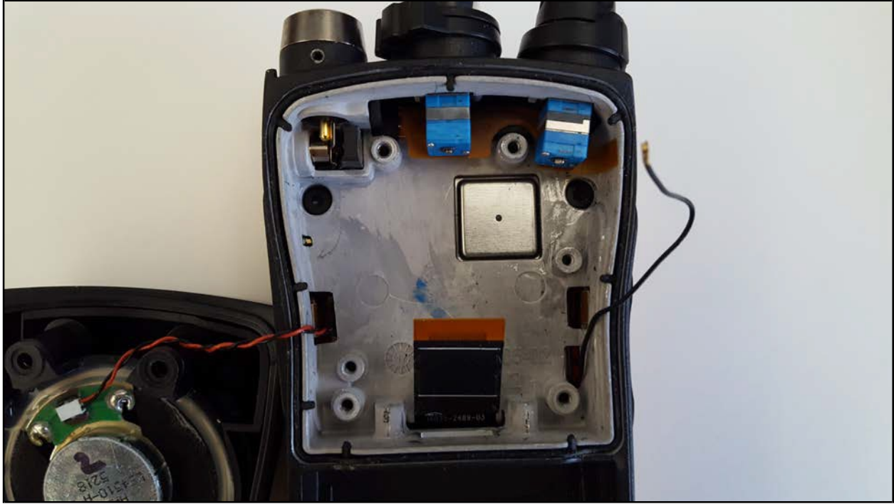
Rear Cover and Expansion Board Removed
