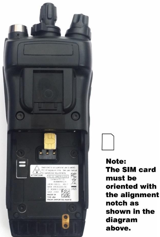
Figure 4-4: SIM Card Installation
