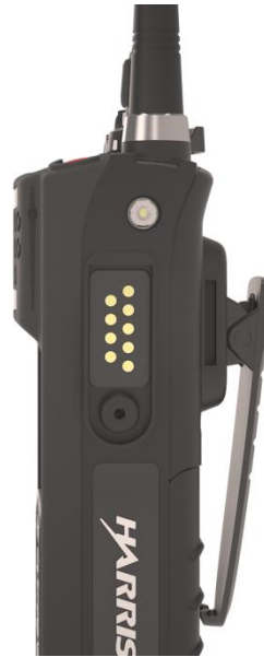
Figure 4-5: Universal Device Connector
