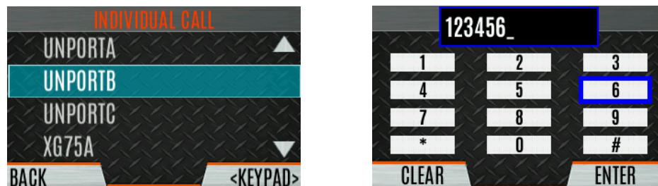
Figure 5-2: Using the Soft DTMF Keypad
