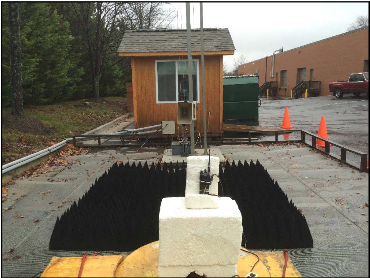
Photograph 1: Radiated Emissions Testing – Front View >1 GHz
