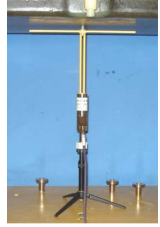
System Performance Check Measurement Setup (IEEE Standard 1528-2003) SPEAG 450 MHz Validation Dipole Setup
