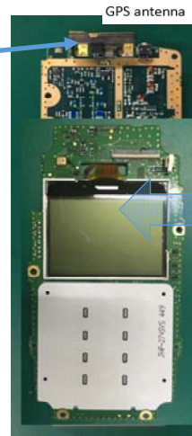
Display board is mounted on top of the RF board
