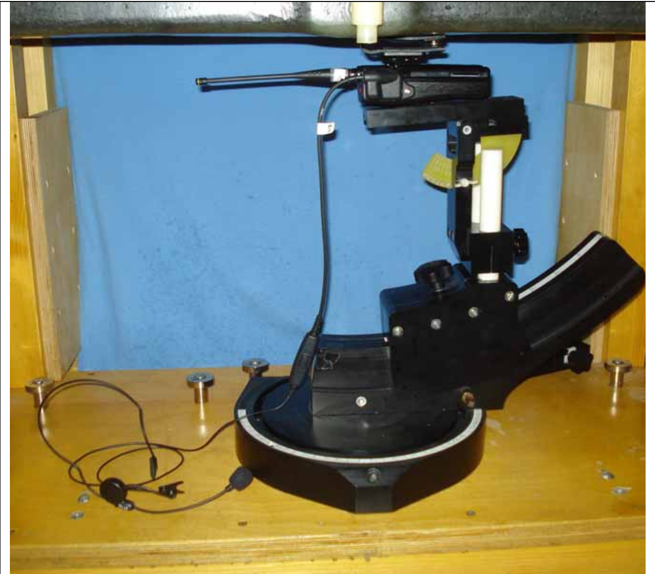
Body-worn Test Setup – Body-worn Acc. 6, Audio Acc. G3a, Antenna 1
