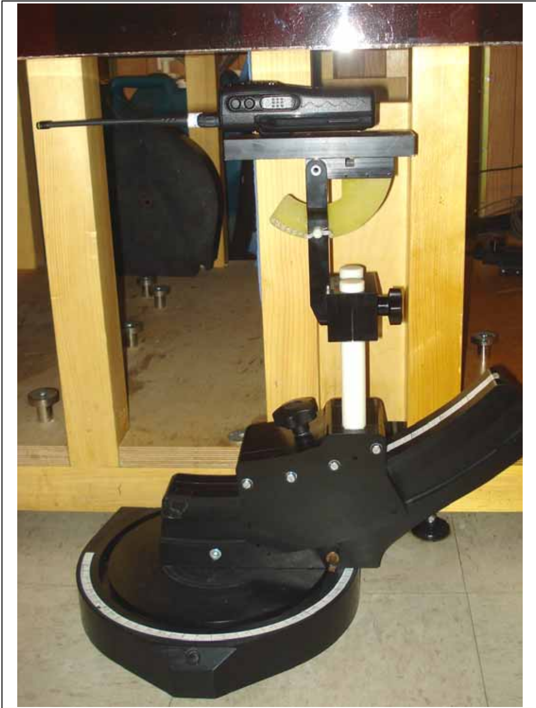
Face-held Test Setup Configuration
