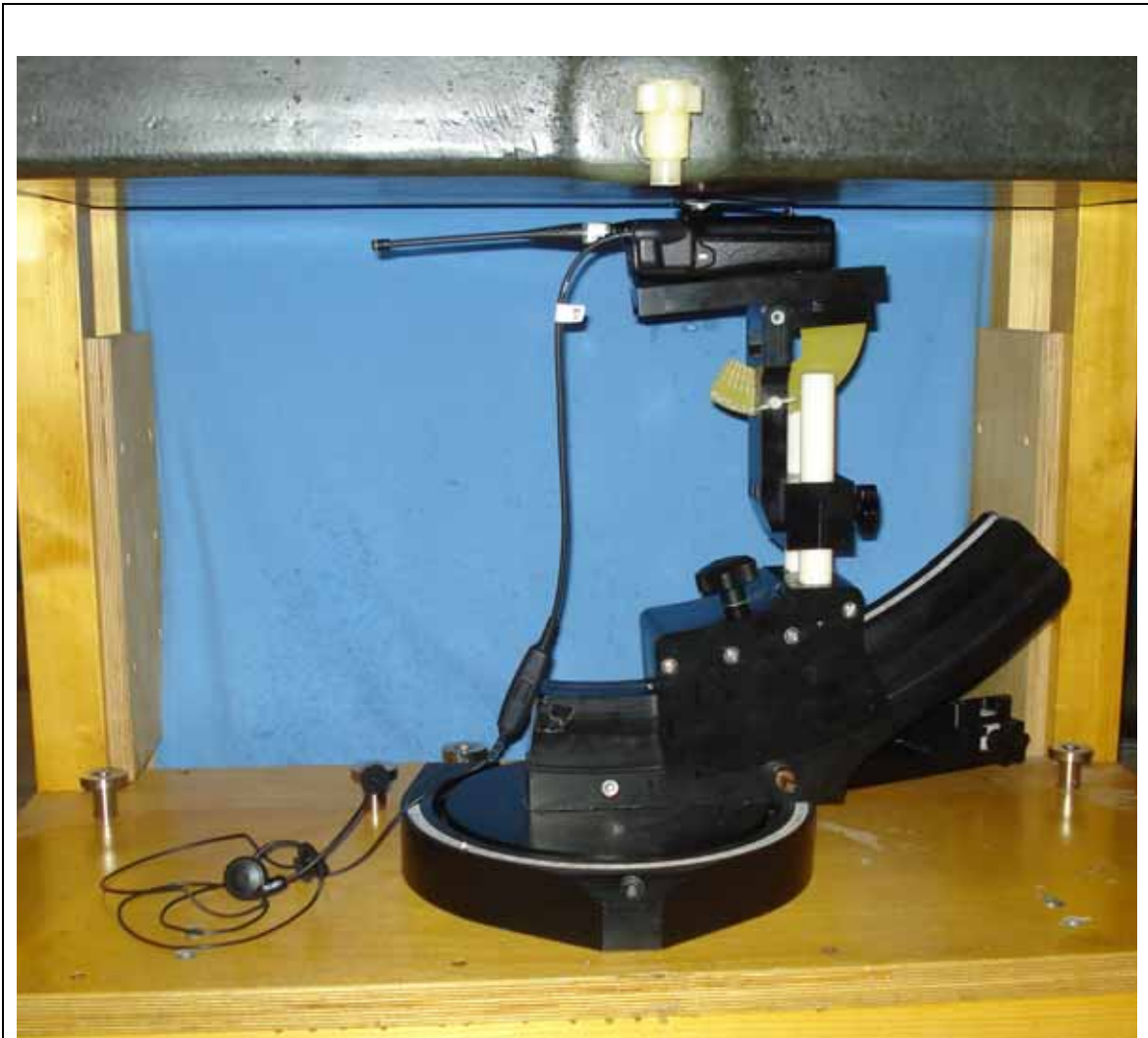
Body-worn Test Setup – Body-worn Acc. 5, Audio Acc. G3a, Antenna 1
