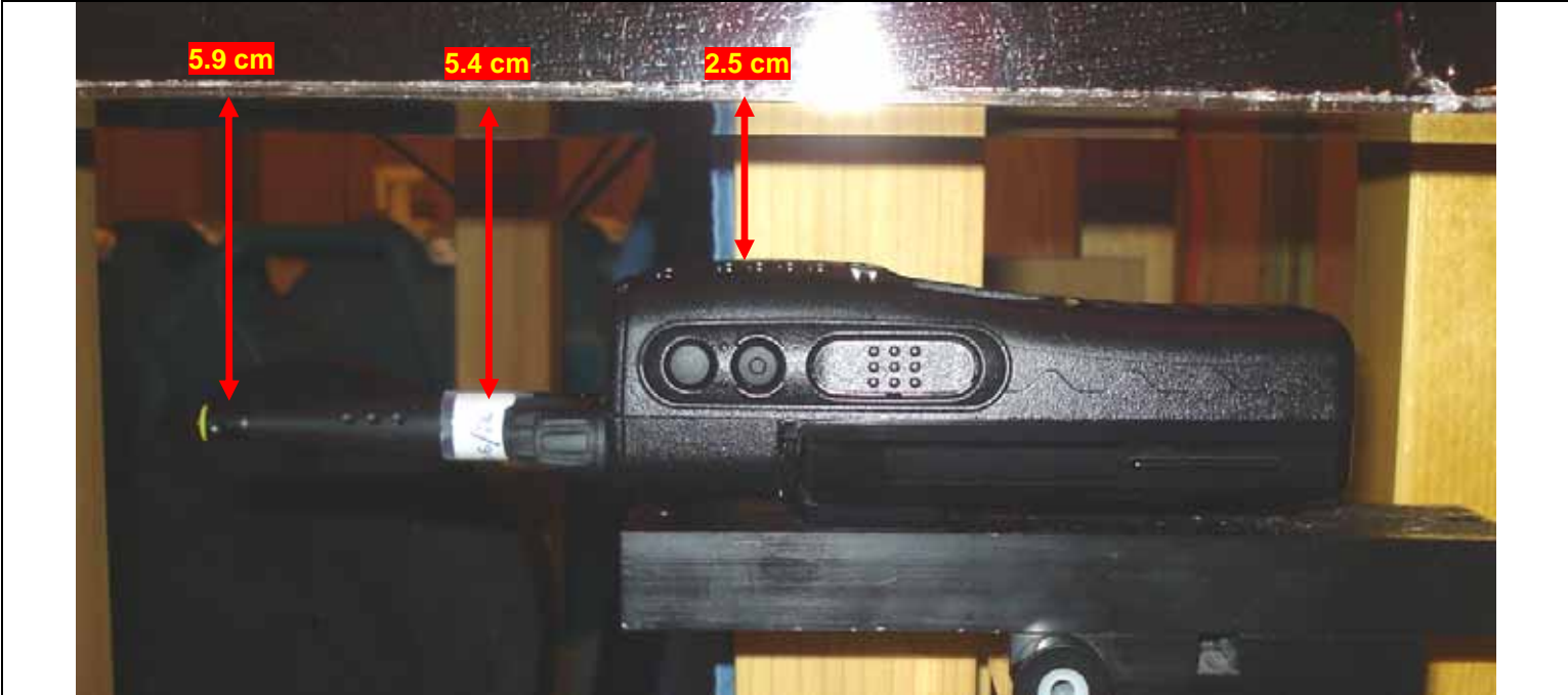
Face-held test setup - Antenna 2
