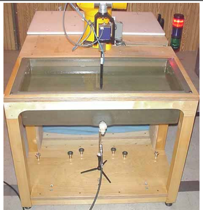
DASY4 Measurement System with Barski Planar Phantom
