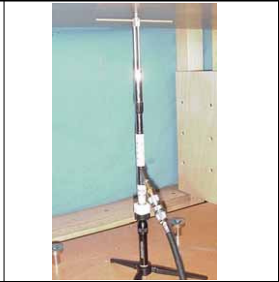
835 MHz SPEAG Validation Dipole Setup
