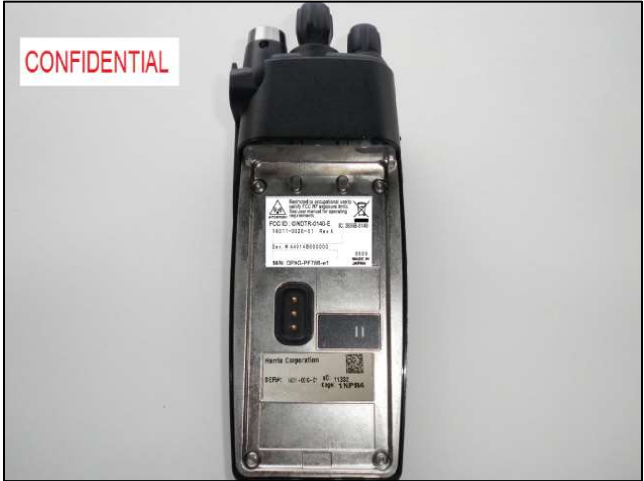
Photograph 3: ID Label Location and RF Safety Label Location
