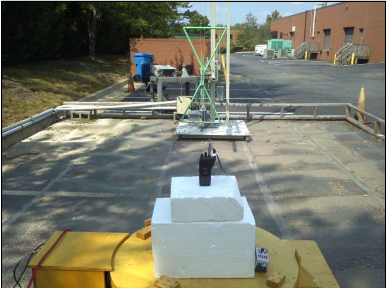
Photograph 4: Radiated Emissions (Spurious/Harmonics) – Front View
