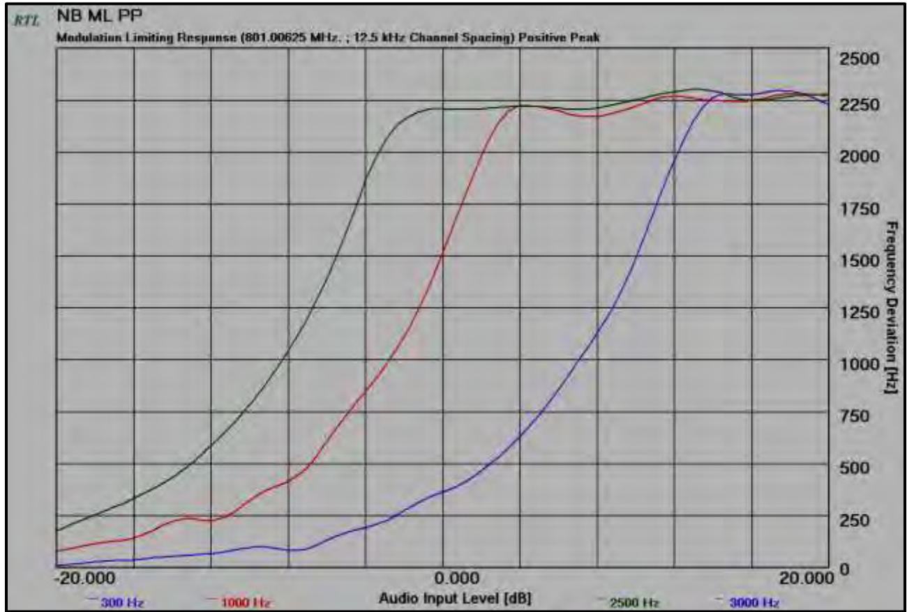
Plot 10-3: Modulation Characteristics – Modulation Limiting – 801.00625 MHz; NB, Positive Peak
