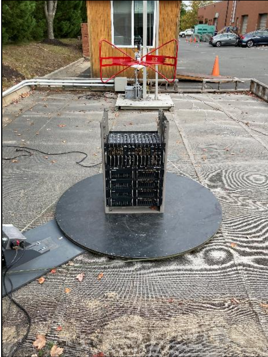
Photograph 1: Radiated Emissions – Front View (Below 1 GHz)
