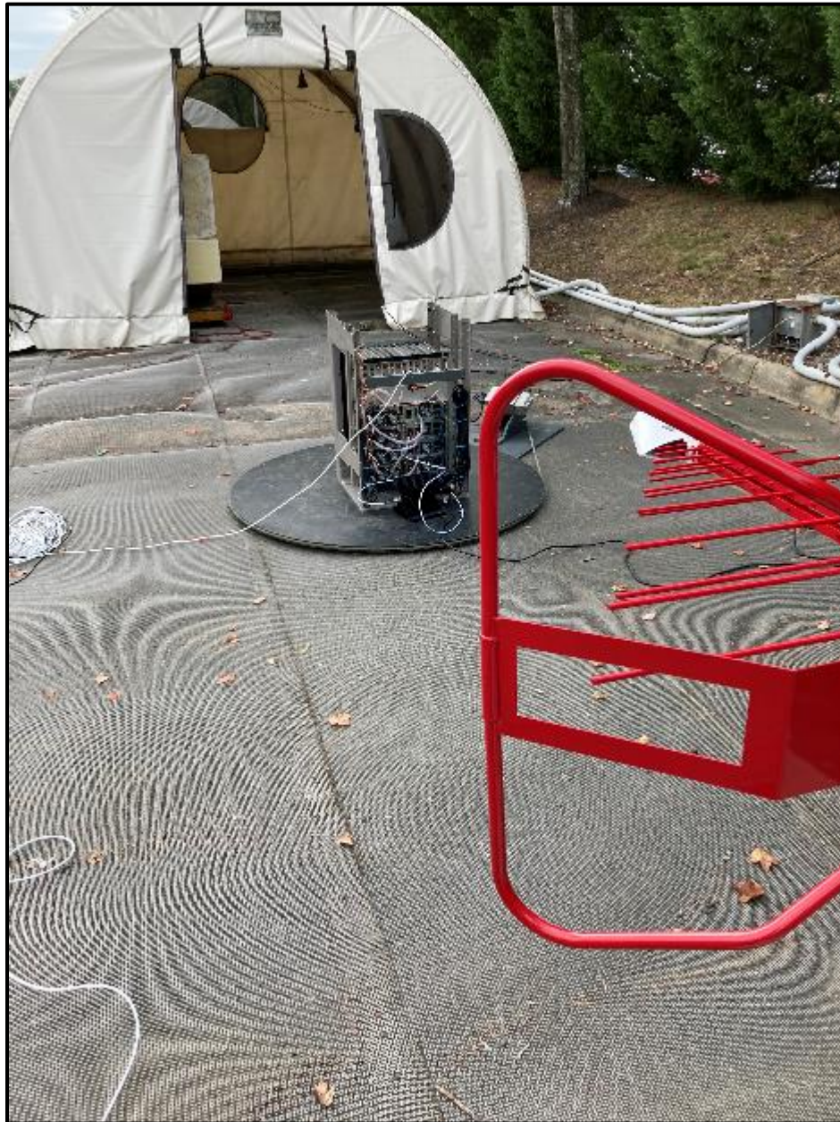
Photograph 2: Radiated Emissions – Back View (Below 1 GHz)
