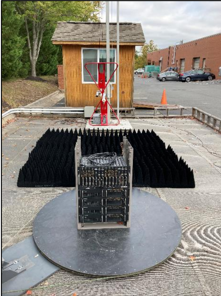
Photograph 3: Radiated Emissions – Front View (Above 1 GHz)
