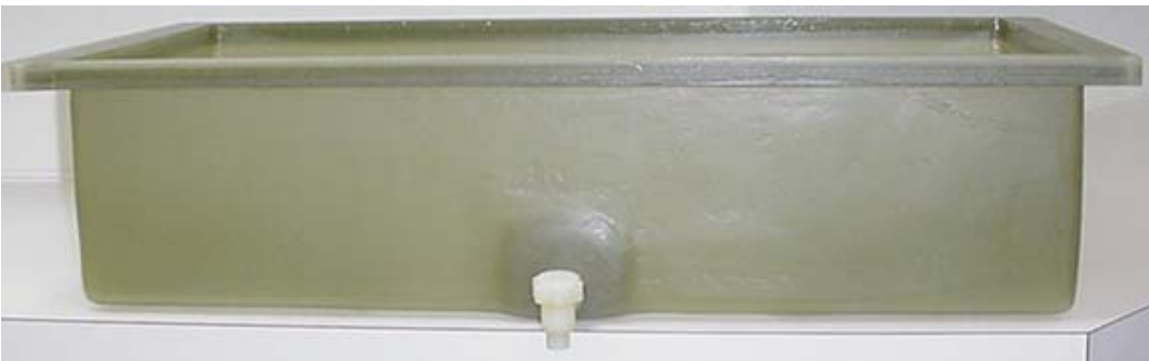
Fiberglass Planar Phantom - Front View
