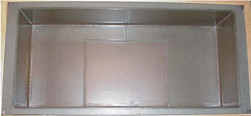
Fiberglass Planar Phantom - Top View
