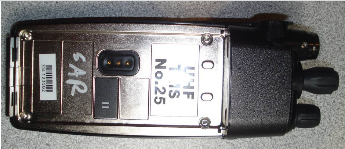
Back of System Radio without battery
