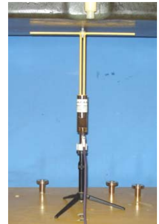
SPEAG 450 MHz Validation Dipole Setup
