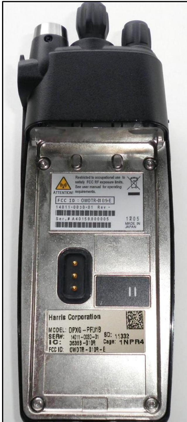
Photograph 4: ID Label Location and RF Safety Label Location
