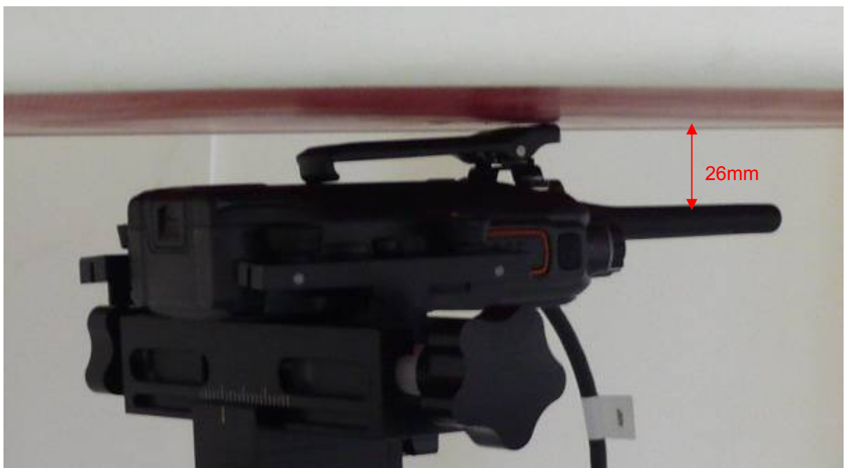
Picture 6: Body-worn with Thinner Battery, Belt and Accessory 1, the front of the EUT towards ground, the distance from EUT Antenna to the bottom of the Phantom is 26mm
