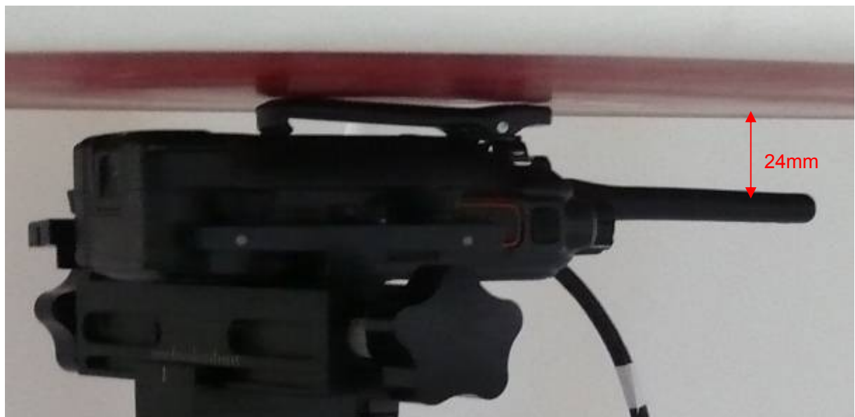
Picture 15: Body-worn with Thicker Battery, Belt and Audio Accessory 2, the front of the EUT towards ground, the distance from EUT Antenna to the bottom of the Phantom is 24mm
