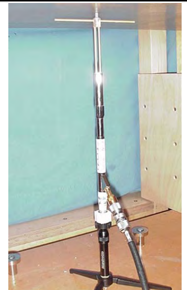
835 MHz SPEAG Validation Dipole Setup
