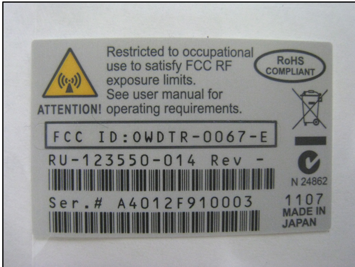
Photograph 4: RF Safety Label Location
