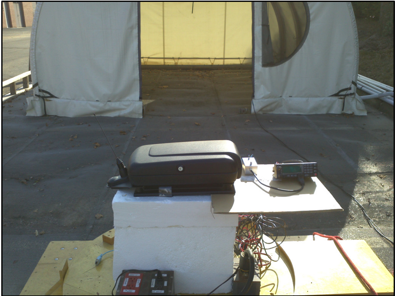
Photograph 1: Radiated Emissions (Spurious/Harmonics) – Front View
