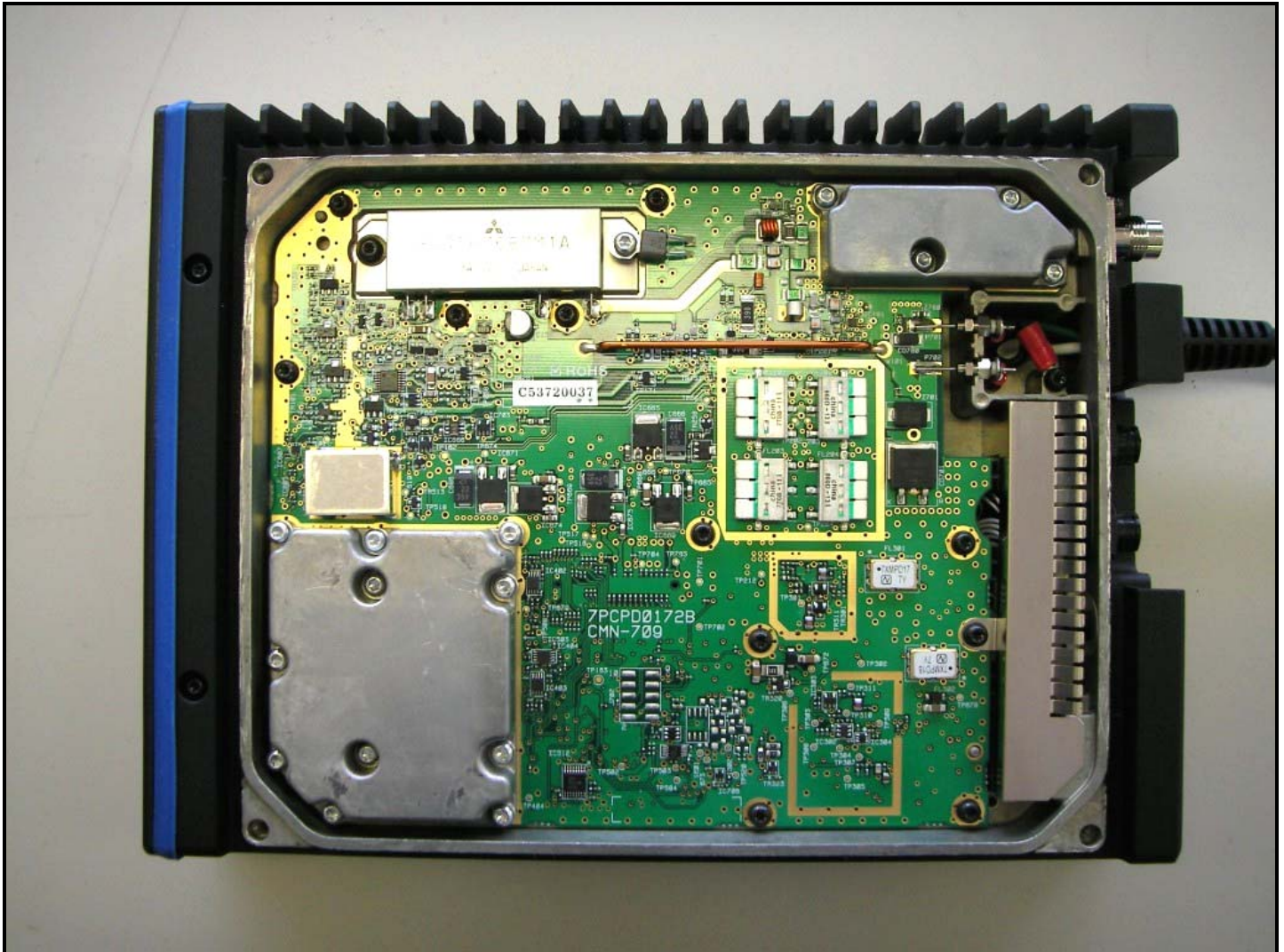
Photograph 3: Bottom Cover and Shield Removed
