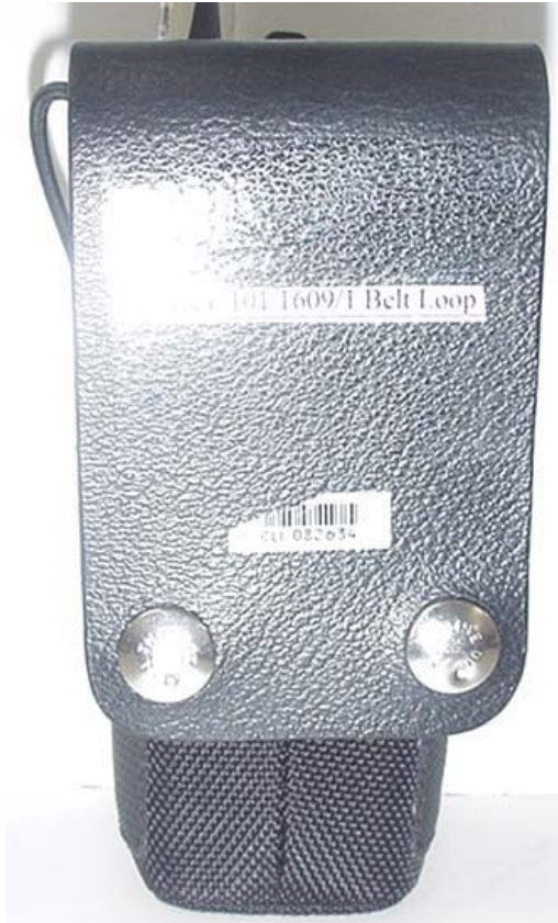
Back of DUT with Nylon Case (P/N: CC-023932-001) and Leather Belt Loop (P/N: KRY 101 1609/1)
