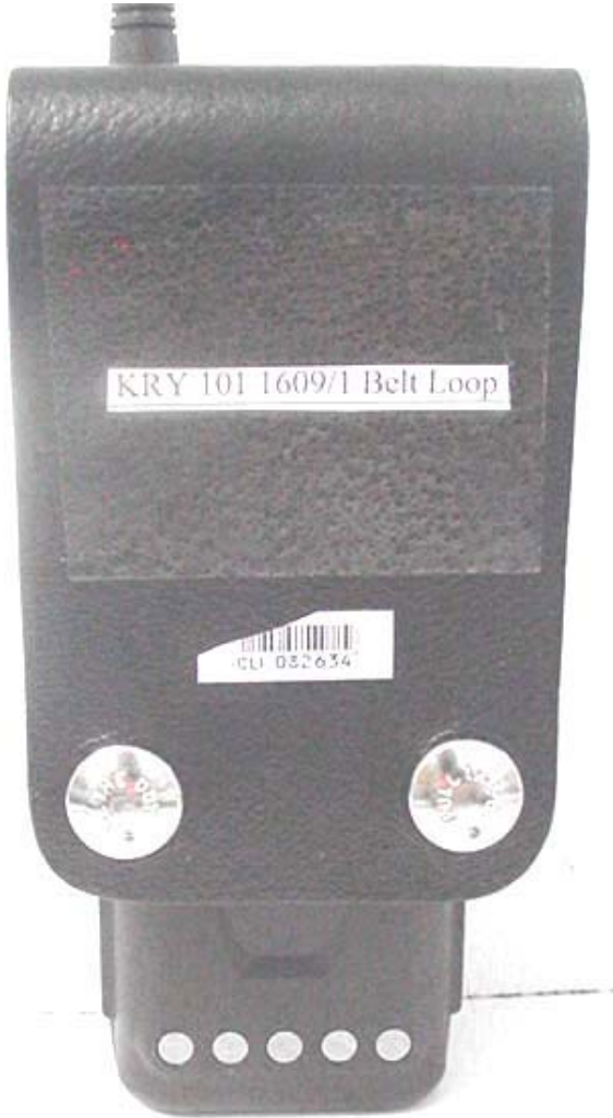
Back of DUT with Leather Belt Loop (P/N: KRY 101 1609/1)
