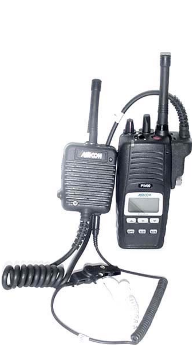
Radio with Speaker-Microphone Antenna Version (P/N: MC-023933-002) and Earphone Audio Accessory (P/N: LS103239V1) Helical Coil Antenna (P/N: KRE 101 1219/10)
