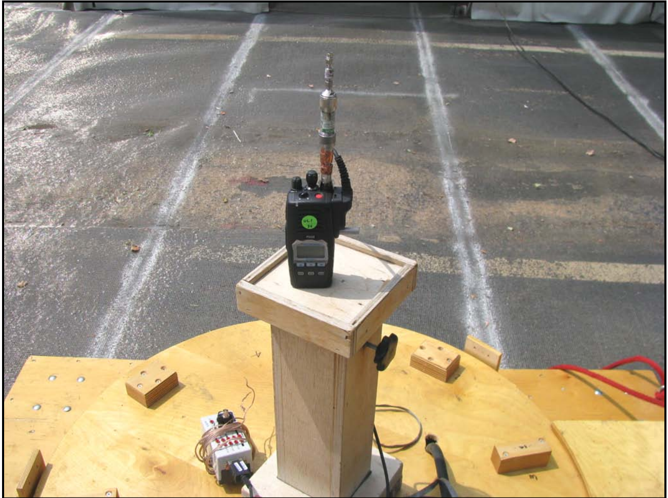
Photograph 1: Radiated Emissions (Front View)
