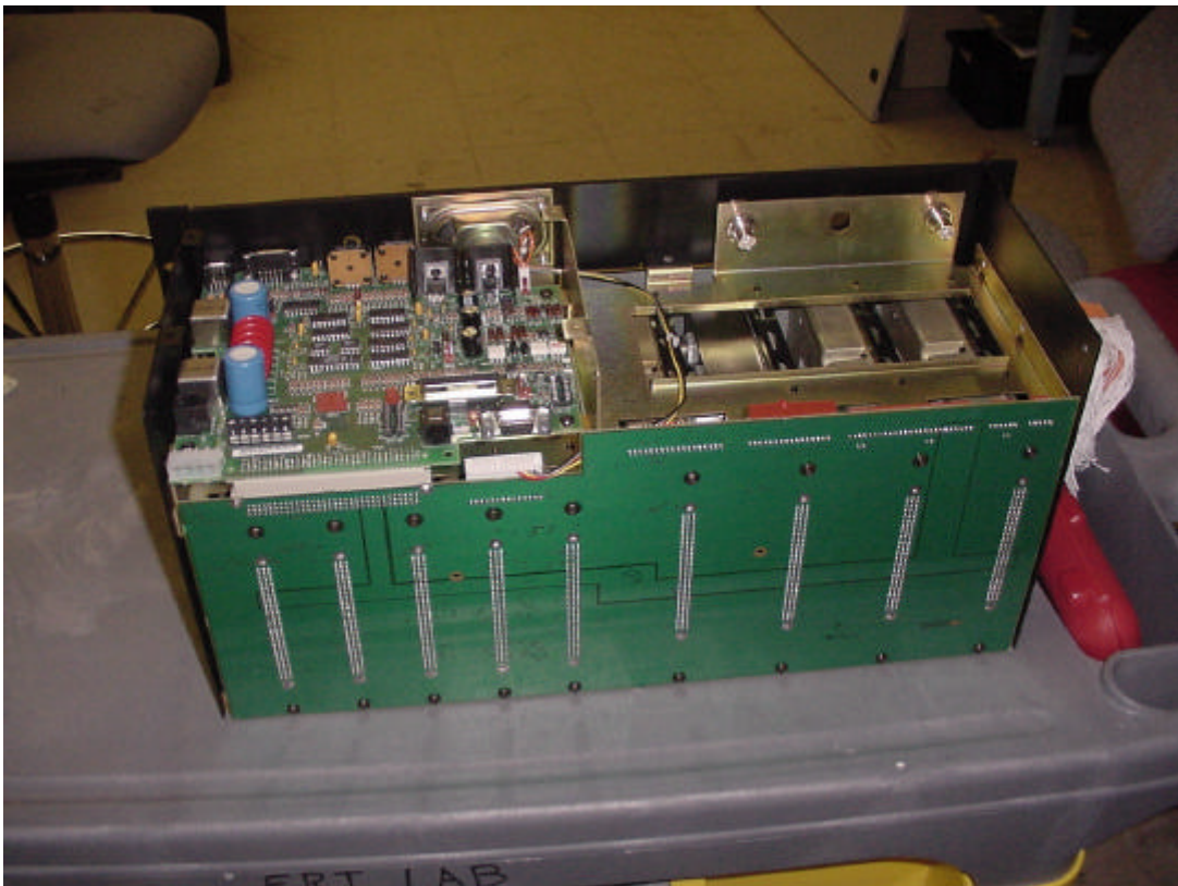
Figure 2 - Mastr III - Rear View
