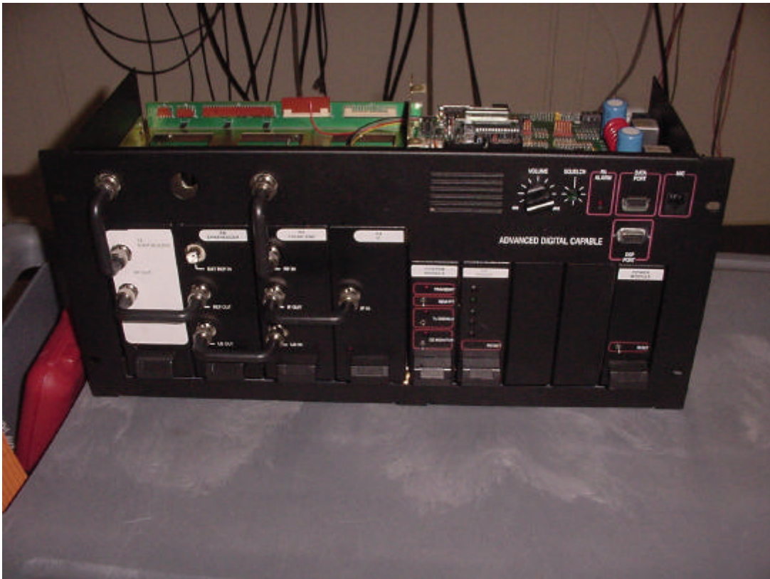
Figure 1 - Mastr III - Front View
