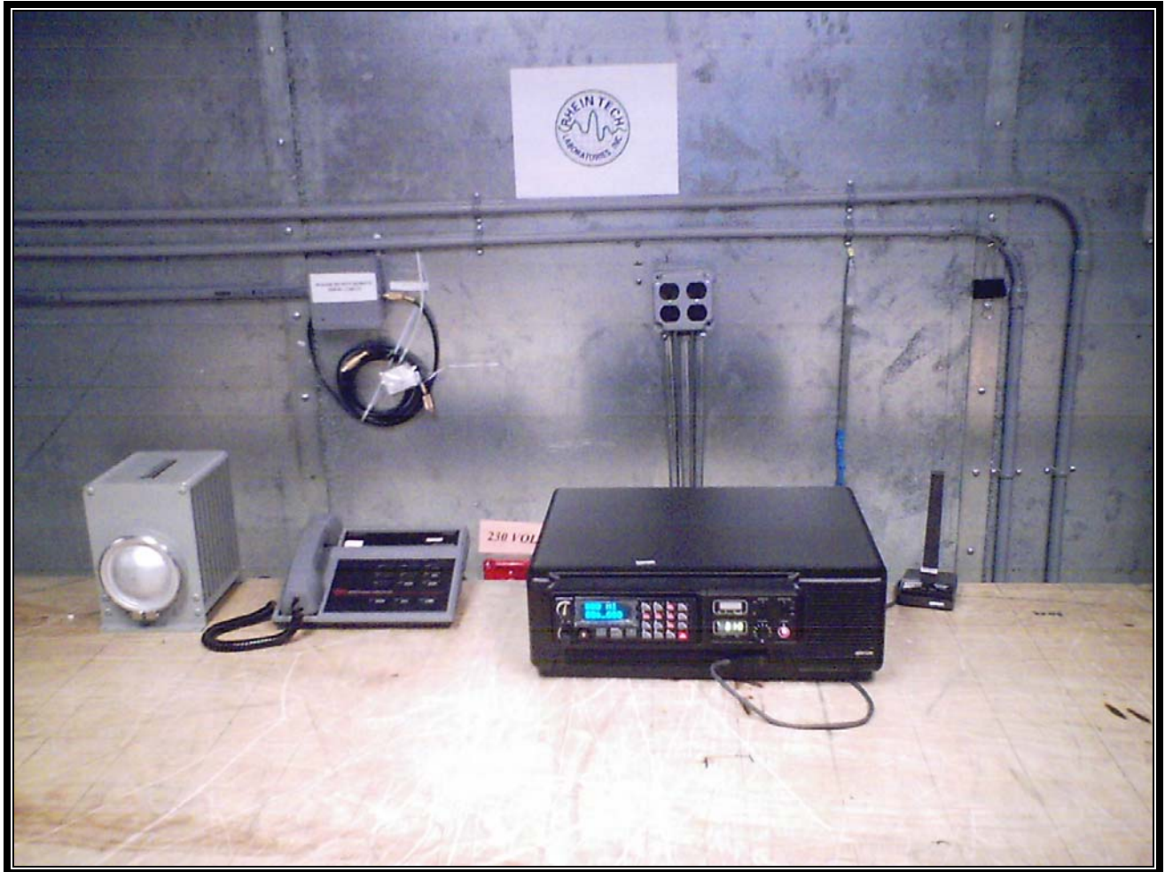
Photograph 7: Conducted Emissions (Front View) Desktop Configuration
