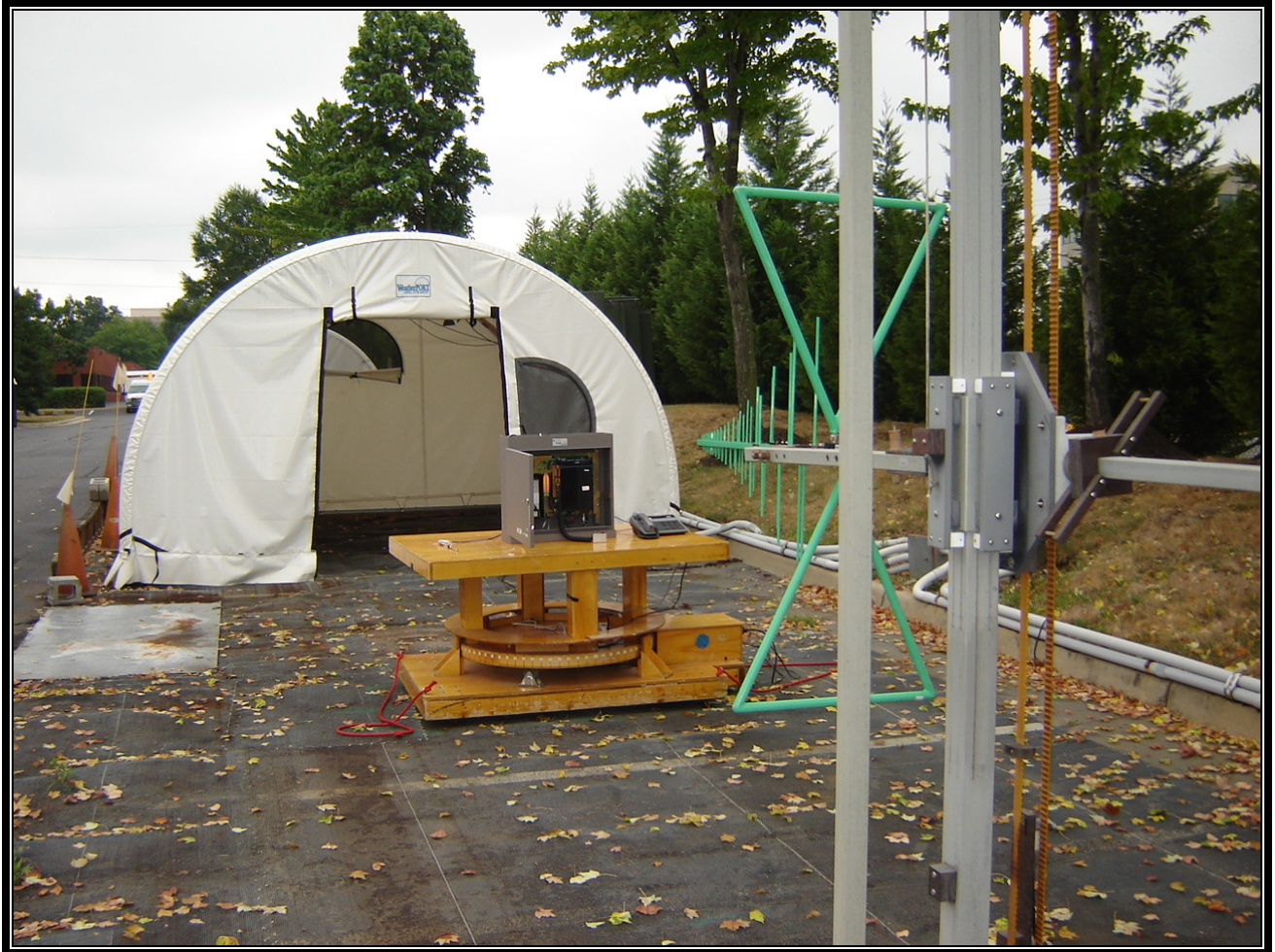
Photograph 1: Radiated Emissions (Front View) Wall Mount Configuration
