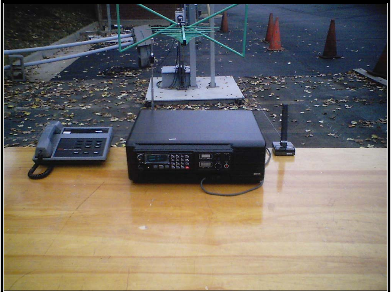
Photograph 3: Radiated Emissions (Front View) Desktop Configuration
