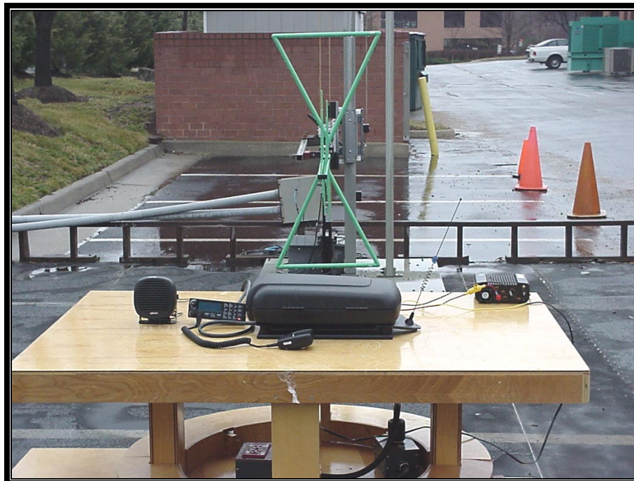
PHOTOGRAPH 4: RADIATED EMISSIONS – MOTORCYCLE CONFIGURATION
