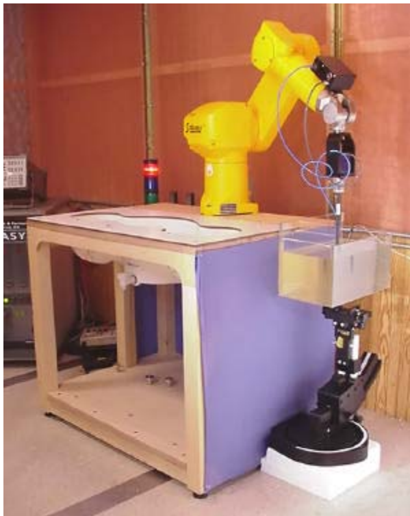
DASY3 SAR Measurement System with Planar Phantom
