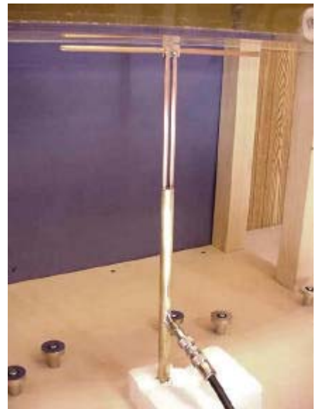
450MHz System Validation Setup Photograph
