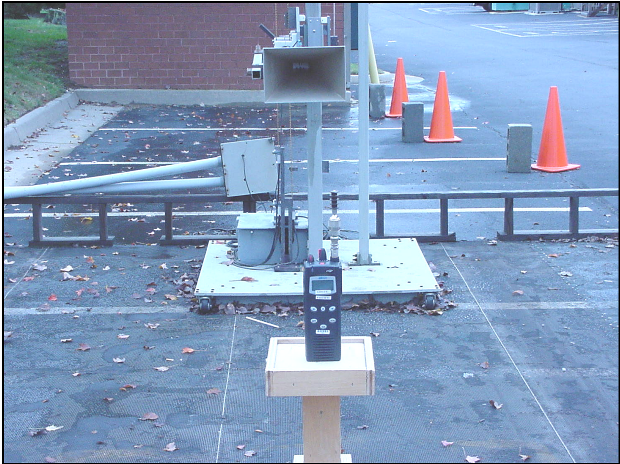
PHOTOGRAPH 7: RADIATED EMISSIONS - FRONT
